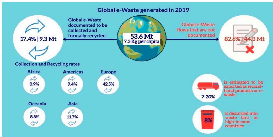
**Figure 2.** Statistics on the amount of E-waste processed formally and informally across the globe [7] (Source: Forti et al., 2020).
