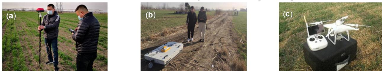
**Figure 6.** Investigation on fissure development characteristics of coal mining working faces. (a) RTK positioning. (b) Geo-radar detection. (c) UAV aerial photo.
