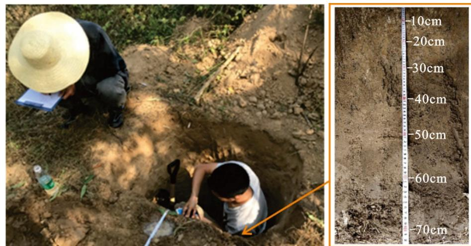
Figure 9. Excavation and sampling of test pit profile.
