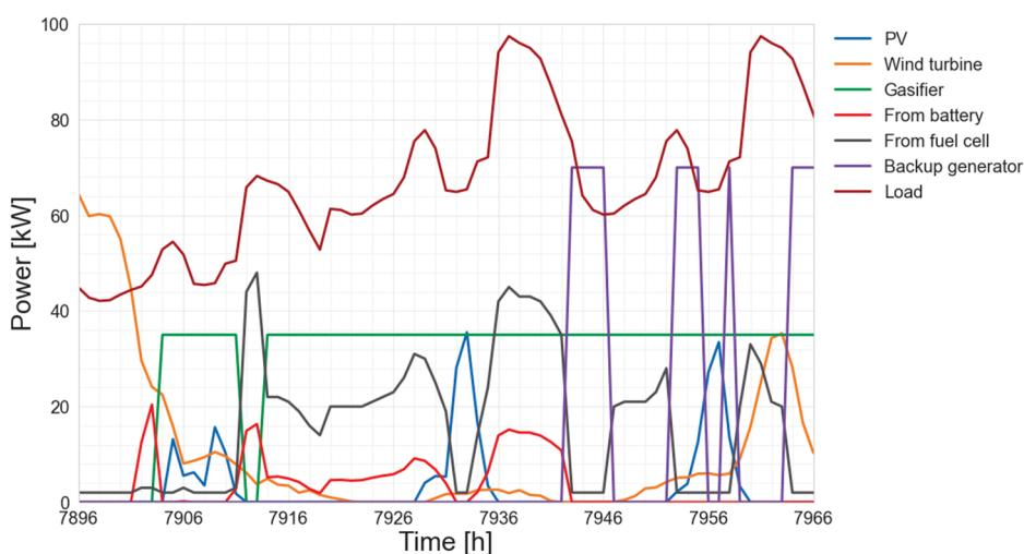
**Figure 15.** Electrical powers of the system for the case of low wind availability period—25–28 November, Gdansk.
