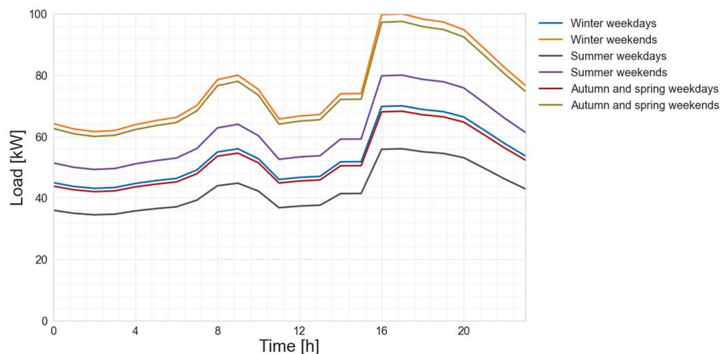
**Figure 3.** Load curve for Gdańsk for different reference days within the year.
