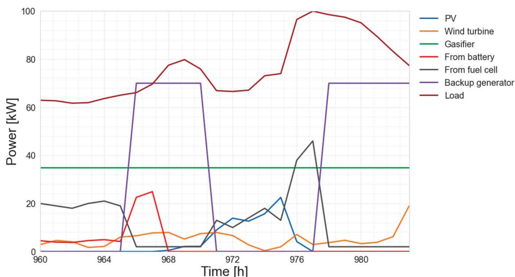
**Figure 14.** Electrical powers of the system for the case of underproduction—selected day of 9 February, Gdansk.
