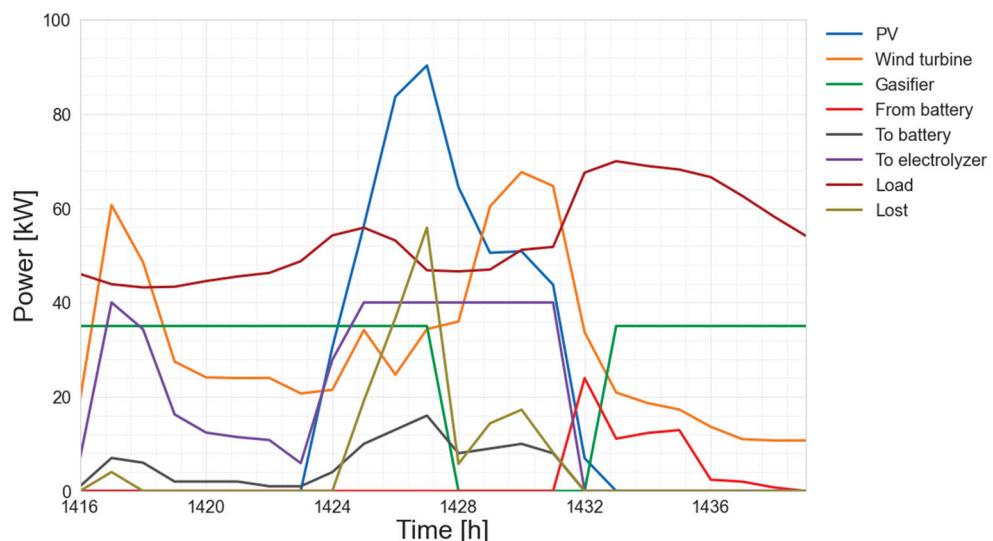
**Figure 12.** Electrical powers of the system for the case of overproduction—selected day of 28 February, Gdansk.
