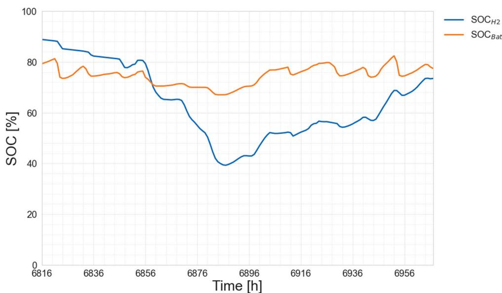
**Figure 8.** Battery and hydrogen state of charge for the case of low wind availability period—11–17 October Agkistro.
