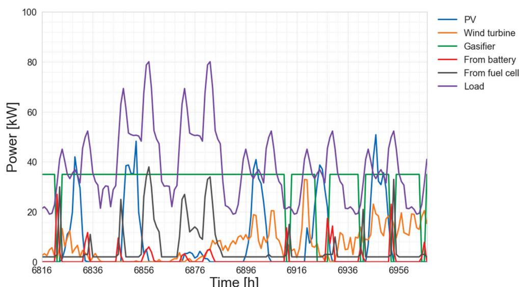
**Figure 7.** Electrical powers of the system for the case of low wind availability period—11–17 October, Agkistro.
