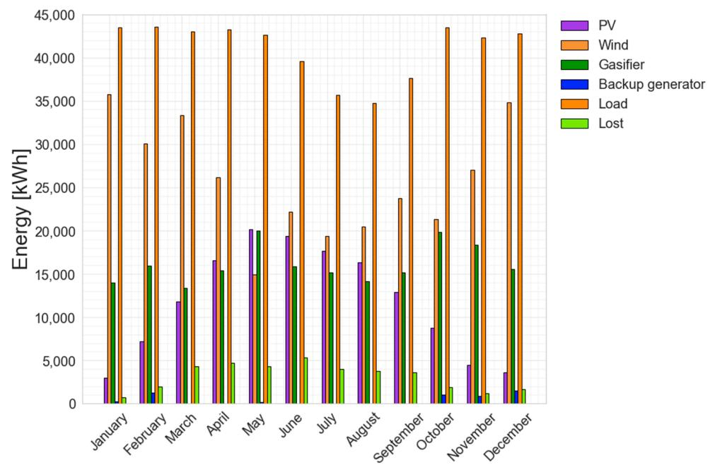
**Figure 17.** Electrical energies of the system, monthly analysis—Gdansk.
