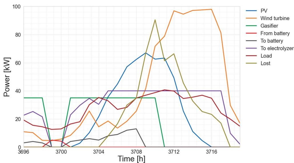
**Figure 4.** Electrical powers of the system in case of overproduction—selected day of 3 June, Agkistro.
