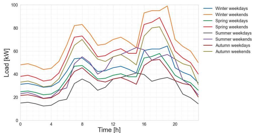
**Figure 2.** Load curve for Agkistro for different reference days within the year.
