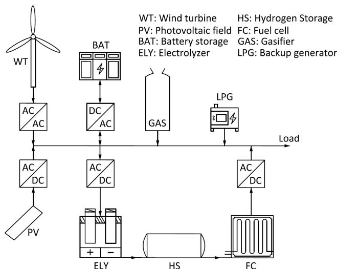
**Figure 1.** Main components of the system and their connection to the AC bus.
