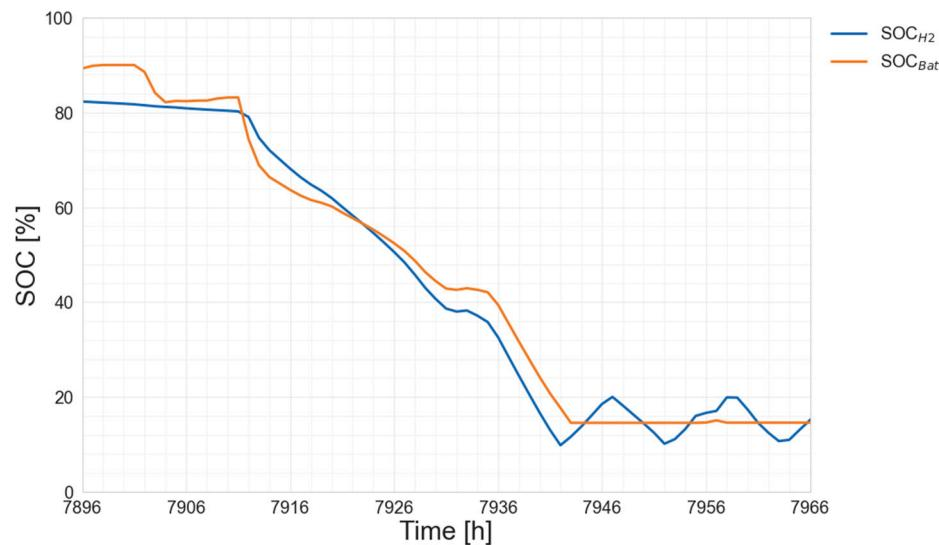
**Figure 16.** Battery and hydrogen state of charge for the case of low wind availability period—25–28 November, Gdansk.
