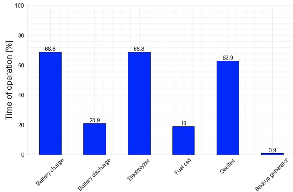
**Figure 19.** The percentage time of use of individual subsystems—Gdansk.
