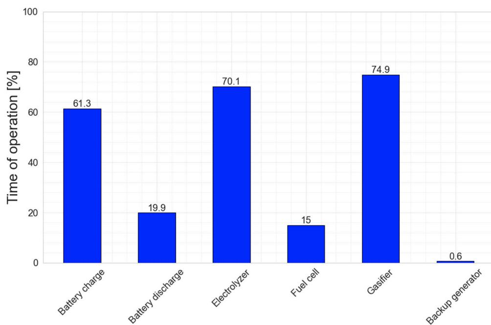
**Figure 11.** The percentage time of use of individual subsystems—Agkistro.
