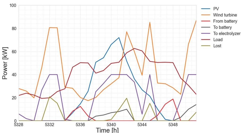
**Figure 5.** Electrical powers of the system for the case of complementary production—selected day of 10 August, Agkistro.
