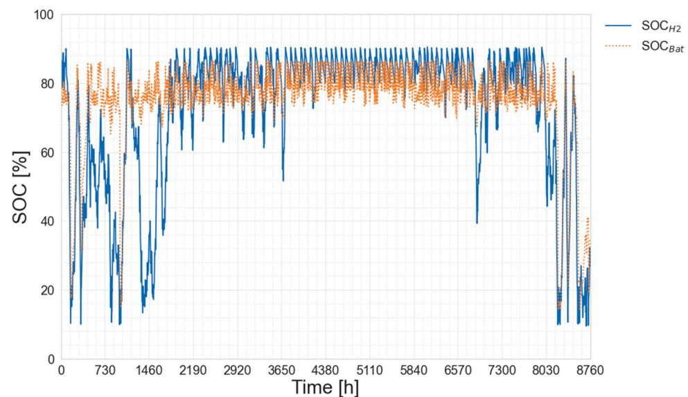
Figure 10. SOC of the energy storage devices—Agkistro.
