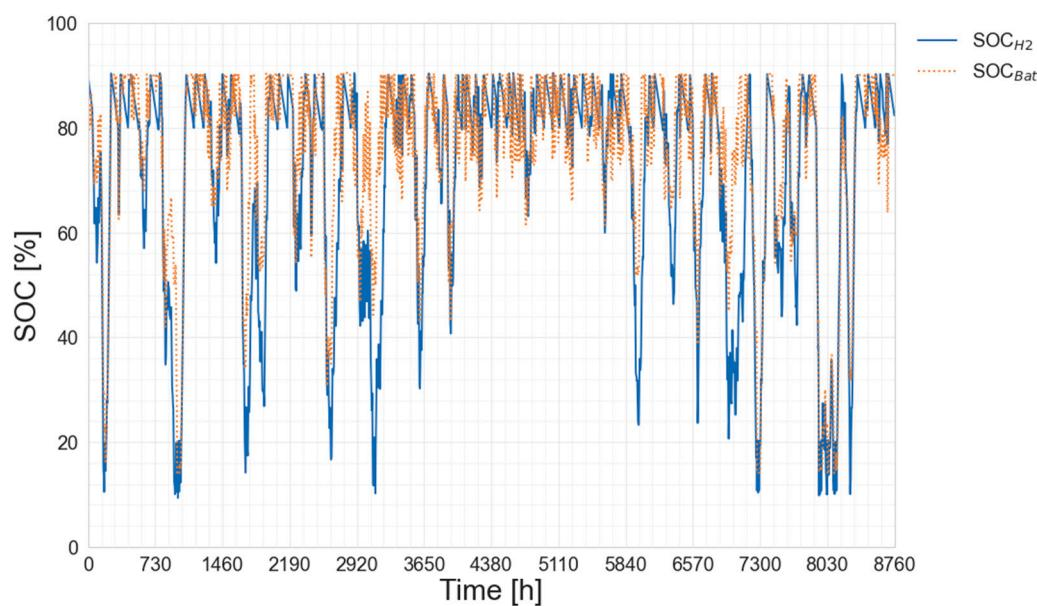
**Figure 18.** SOC of the energy storage devices—Gdansk.
