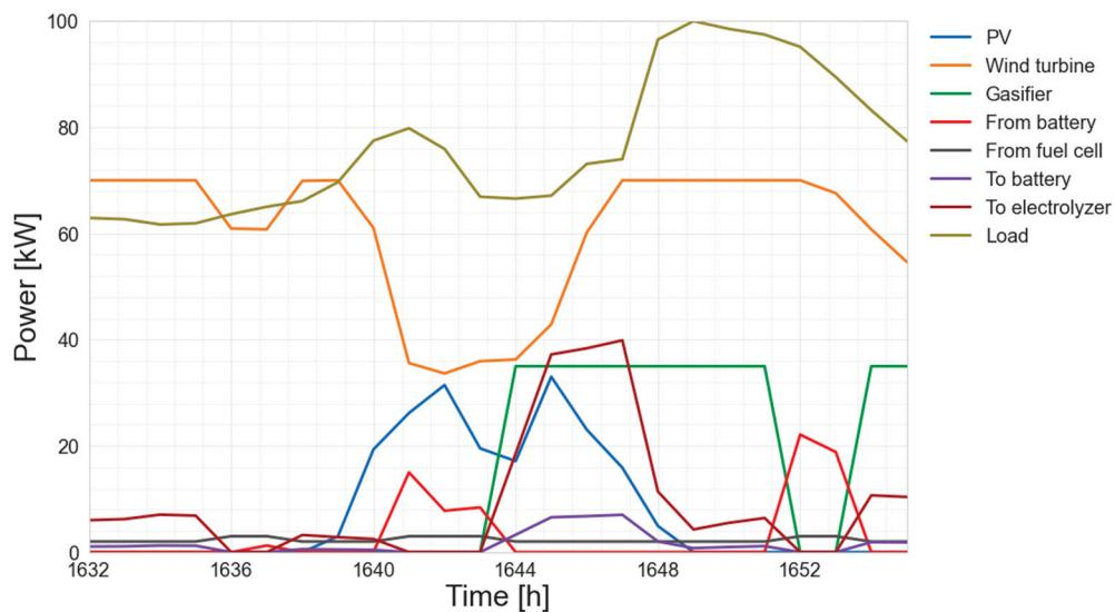
**Figure 13.** Electrical powers of the system for the case of complementary production—selected day of 9 March, Gdansk.
