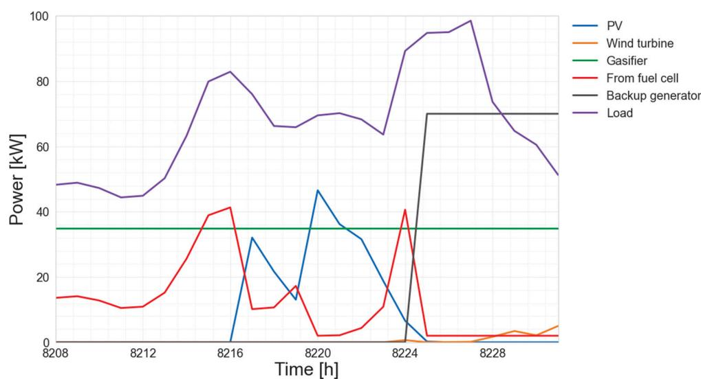
**Figure 6.** Electrical powers of the system for the case of underproduction—selected day of 8 December Agkistro.
