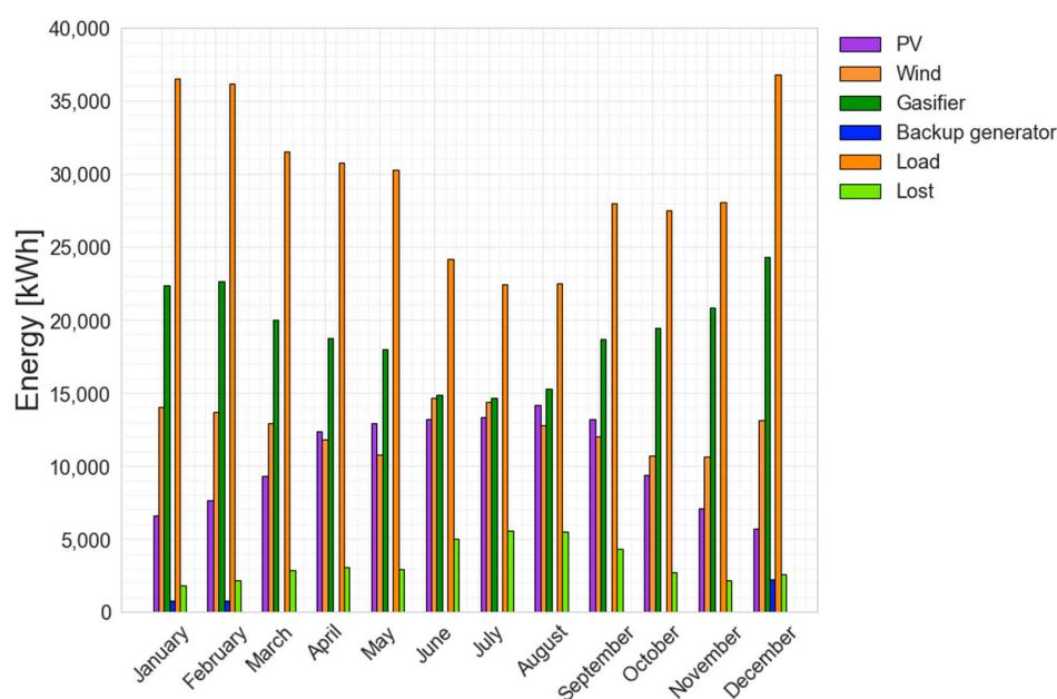
Figure 9. Electrical energies of the system, monthly analysis—Agkistro.
