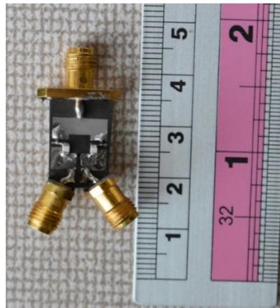
**Figure 15.** Fabricated photo of the proposed 900 MHz divider with a 92% size reduction.
