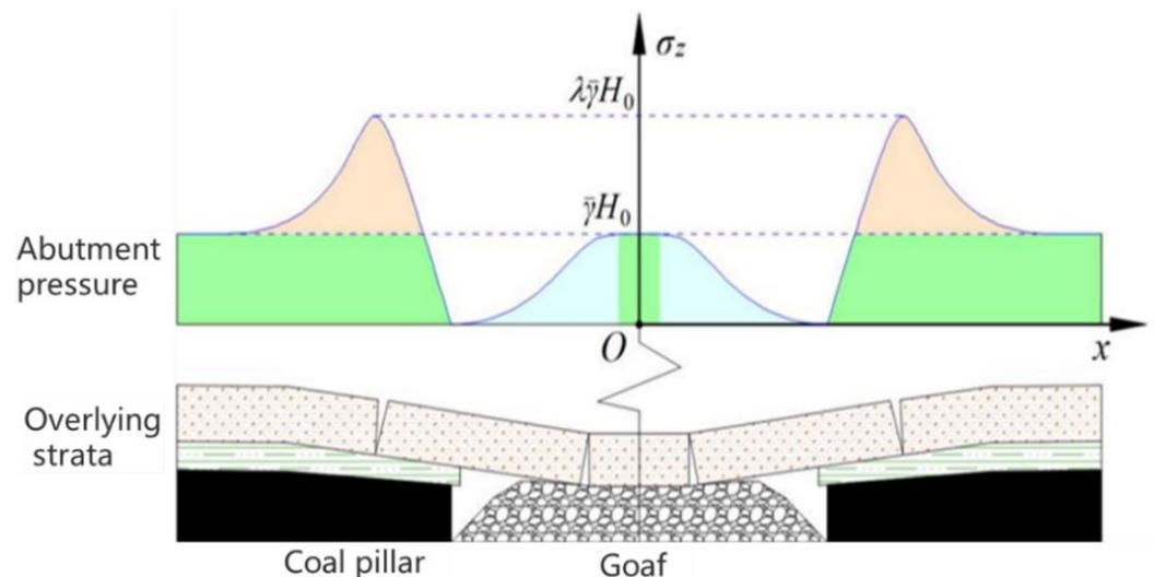
**Figure 1.** Distribution of abutment pressure in surrounding rock of mining stope [21].
