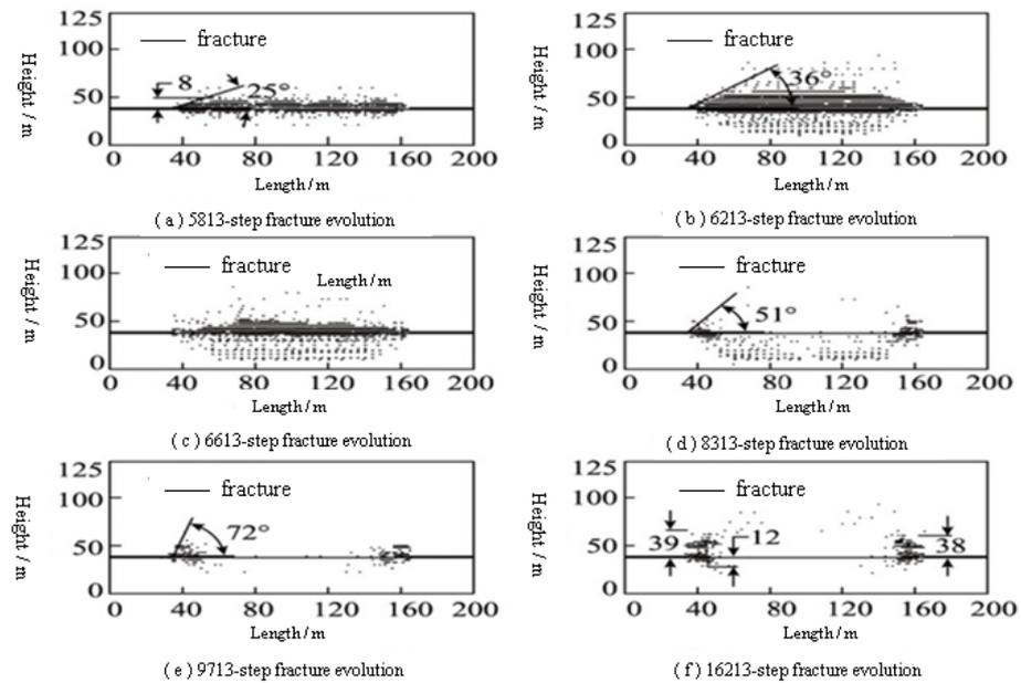
Figure 5. Fracture evolution process in different mining steps [27].
