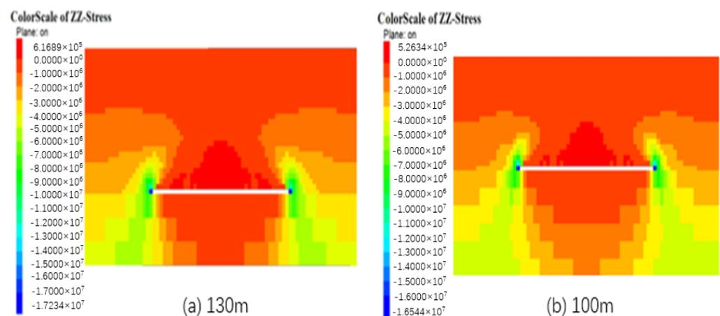
**Figure 3.** Vertical-stress distribution around goaf area under different mining depths [24].
