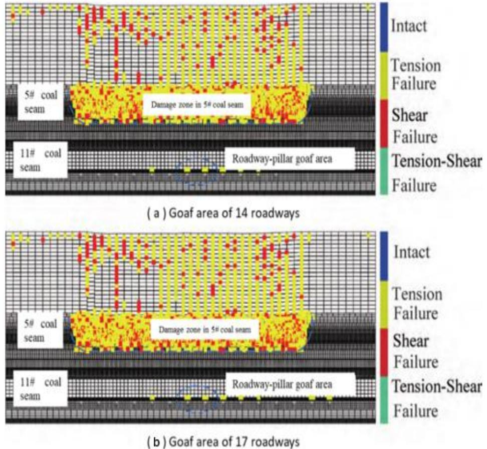
Figure 6. Evolution of mining fractures in mining stope [28].
