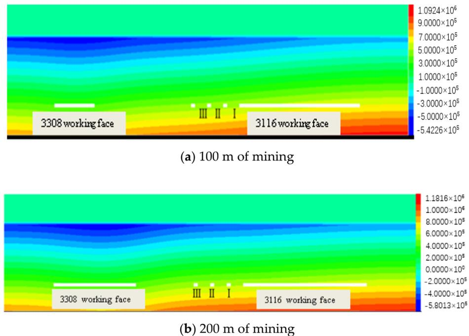
**Figure 9.** Pore-water-pressure distribution in 3308 mining working face [36].
