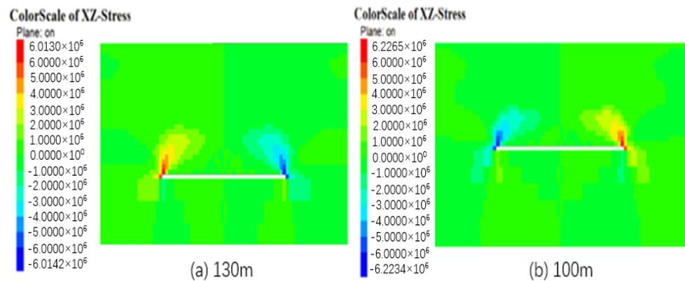
**Figure 4.** Shear-stress distribution around goaf area under different mining depths [24].
