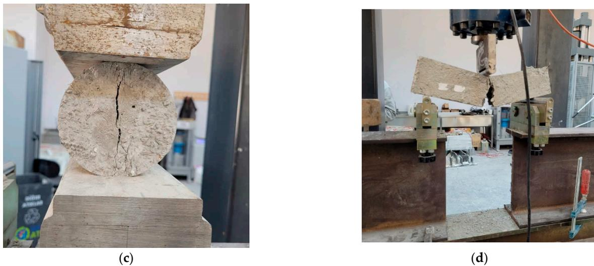
**Figure 3.** Mechanical test setupsL (a) compressive strength, (b) compressive strength, (c) splitting tensile test and (d) bending test.
