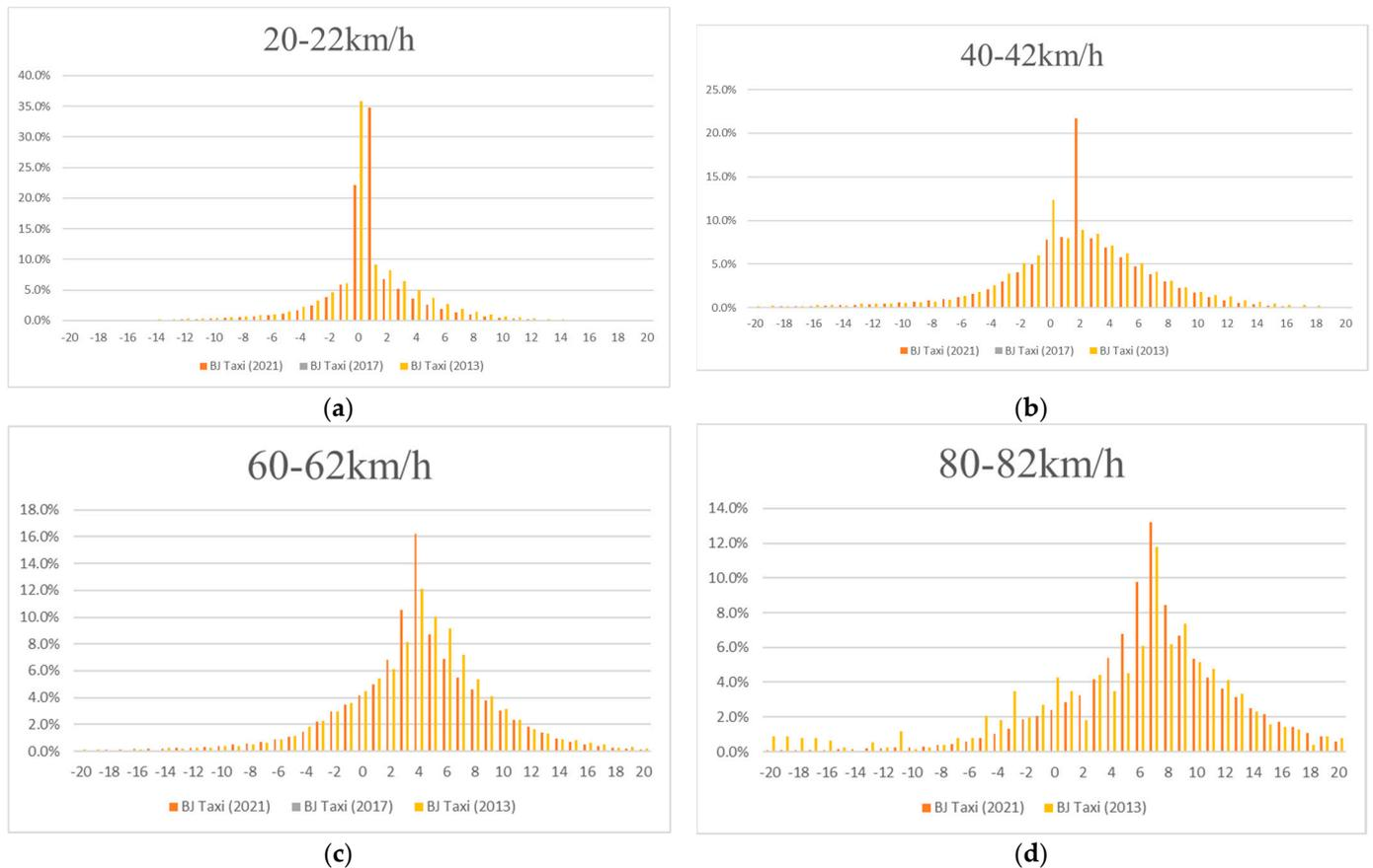
**Figure 4.** Distribution of VSP bin at the mean velocity interval. (a) VSP distributions of Op mode ID BJ taxi between 20 km/h and 22 km/h. (b) VSP distributions of Op mode ID BJ taxi between 40 km/h and 42 km/h. (c) VSP distributions of Op mode ID BJ taxi between 60 km/h and 62 km/h. (d) VSP distributions of Op mode ID BJ taxi between 80 km/h and 82 km/h.
