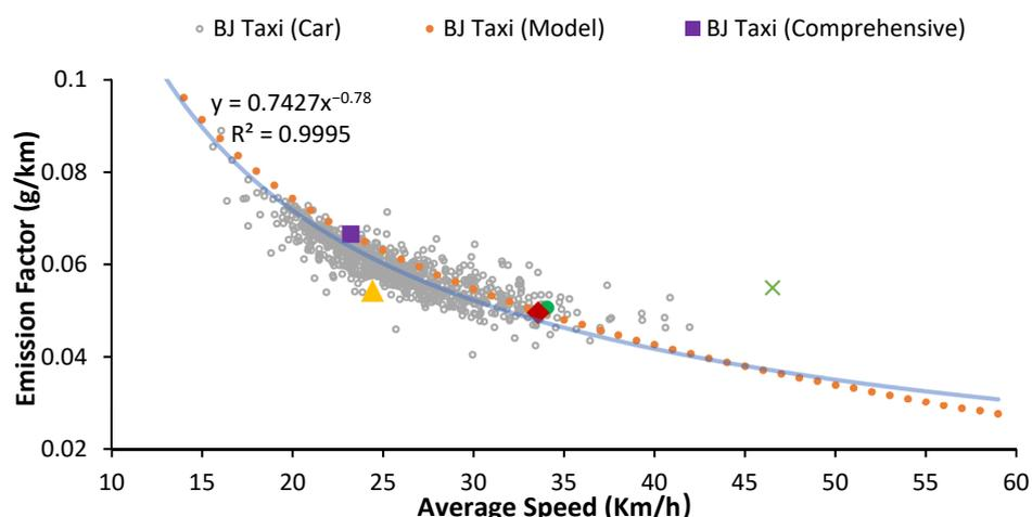
Figure 8. NOx emission factors of average speed, single car, and correction curve in BJ taxi and typical driving cycles.
