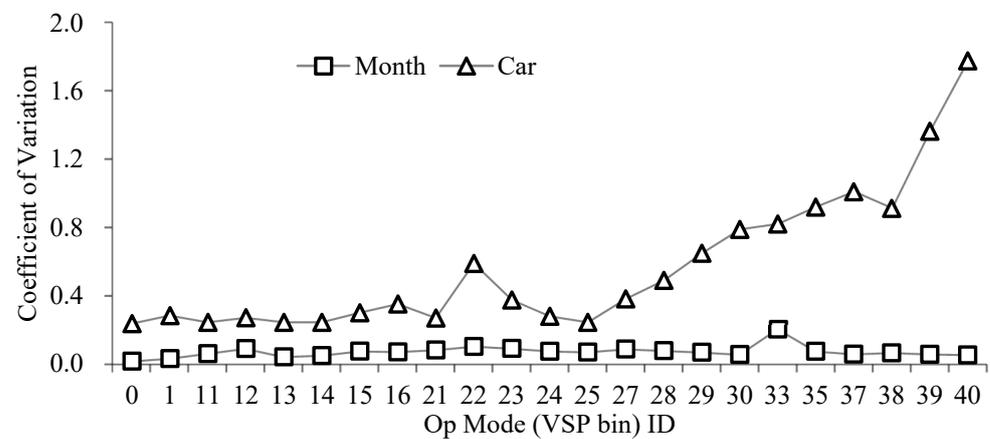
**Figure 5.** Coefficient of Variation in Op Mode divided by month and car.
