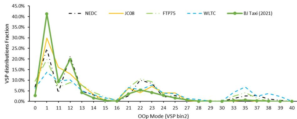
Figure 7. VSP distributions of typical driving cycle.
