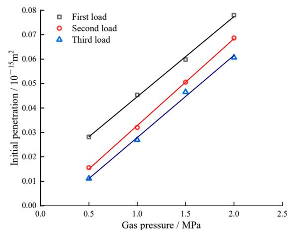
**Figure 10.** Variation trend of initial permeability of coal samples under different gas pressures.
