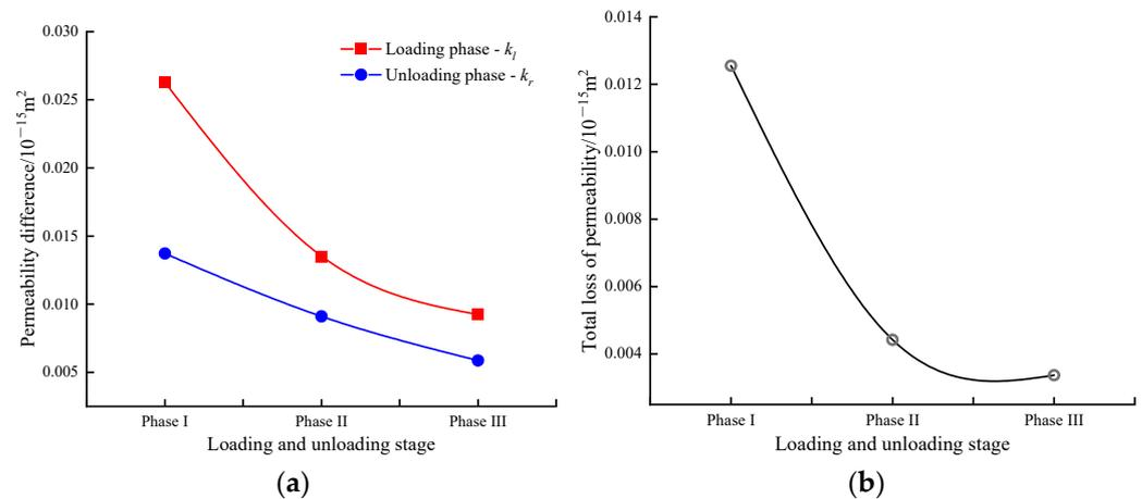
**Figure 8.** Permeability difference: (a) Permeability difference at each loading (unloading) stage; (b) Permeability difference at the minimum confining pressure in the same stage.
