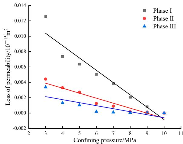
**Figure 9.** Permeability loss of coal samples at different confining pressures.
