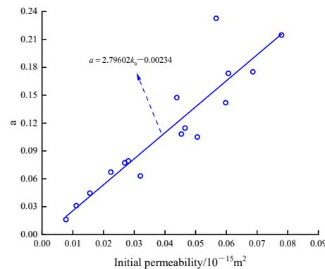
**Figure 7.** Relationship between fitting coefficient  $a$  and initial permeability.
