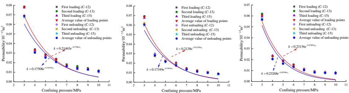
Figure 6. Permeability of coal sample when gas pressure is 2 MPa.
