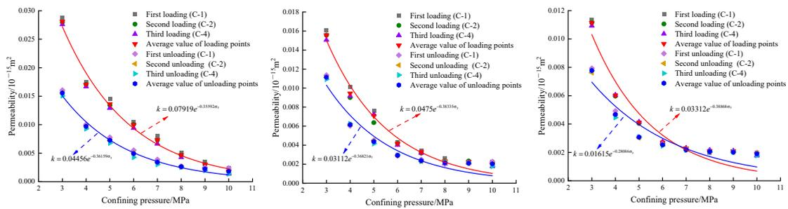
Figure 3. Permeability of coal sample when gas pressure is 0.5 MPa.
