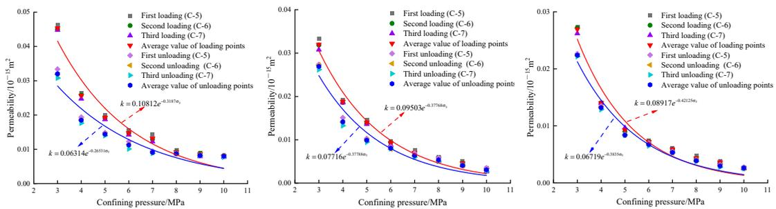
Figure 4. Permeability of coal sample when gas pressure is 1 MPa.
