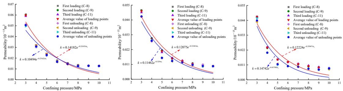
Figure 5. Permeability of coal sample when gas pressure is 1.5 MPa.
