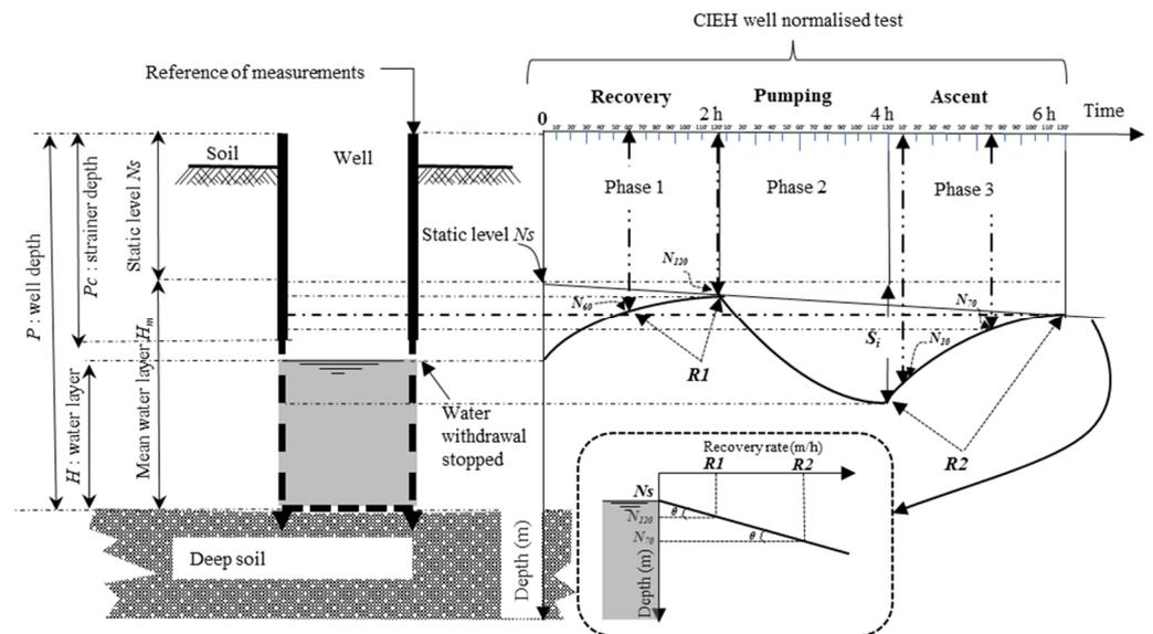
**Figure 2.** CIEH well-pumping test principle and variables.
