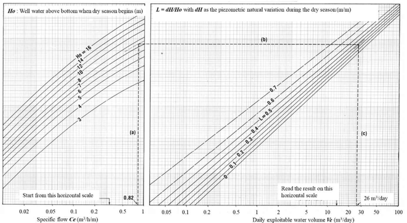
Figure 3. Abacus N3. Determination of the well’s daily exploitable water  $V_e$ .
