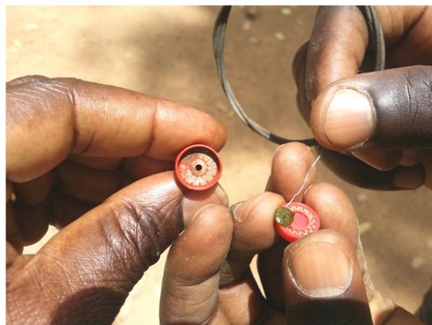
**Figure 7.** Dripper clogged by disk-shaped algae despite filtration.
