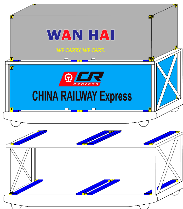
Figure 3. Structural drawing of the new special articulated flat car for double-stack container trains.
