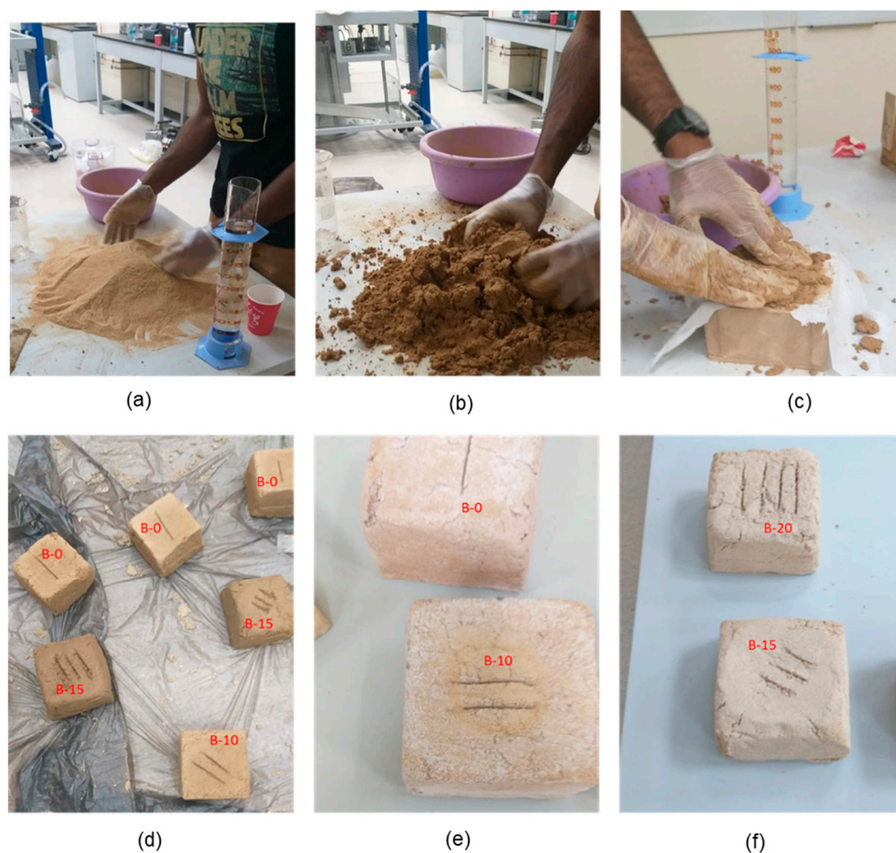
Figure 3. Laboratory procedure for porous clay bricks made of soil and sawdust for this study, (a) mixing soil and sawdust waste, (b) dough-making process by adding water, (c) casting dough into a wooden mold, (d) bricks after sun/oven drying, (e,f) bricks after completing the baking process.
