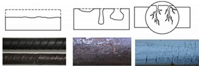
**Figure 8.** Illustration of corrosion in rock bolts, from left to right: uniform corrosion, pitting corrosion and stress corrosion, adapted from Xu and Gutierrez [45], Copyright ©2022, with permission from Elsevier, License No. 5344140552087.
