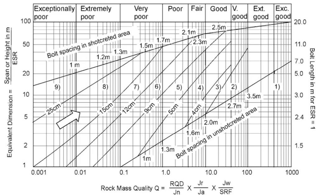
**Figure 17.** Chart of the Q-systems of rock support (From Barton [162], Copyright©2022, with permission from Elsevier, License No. 5378160017237).
