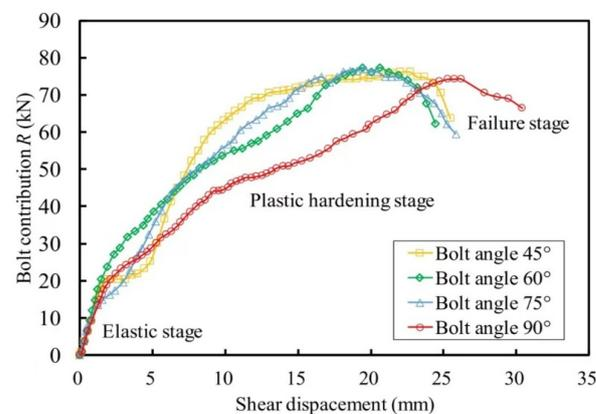
**Figure 12.** Comparison of shear resistance and shear displacement for different installation angle of rock bolt, reprinted from Li et al. [152], Copyright ©2022, with permission from Elsevier, License No. 5344141390457.
