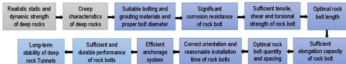
**Figure 20.** Steps leading to the design of rock bolts that can have sufficient and durable performance and therefore the ability to properly ensure the long-term stability of deep rock tunnels.
