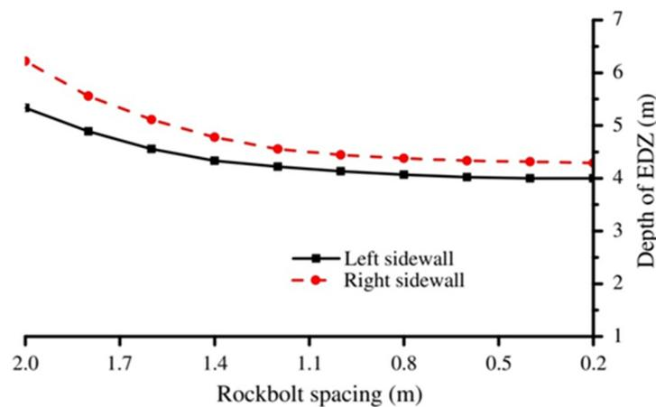
**Figure 11.** Effects of Rock Bolt Spacing on the Extent of Excavation Damaged Zones of Rock Surrounding Tunnels, reprinted from Feng et al. [138], Copyright ©2022, with permission from Springer Nature, License No. 5344180177286.
