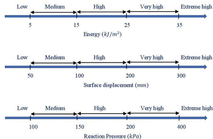
Figure 18. Ground demand in terms of energy, surface displacement and pressure, adapted from [14,33].
