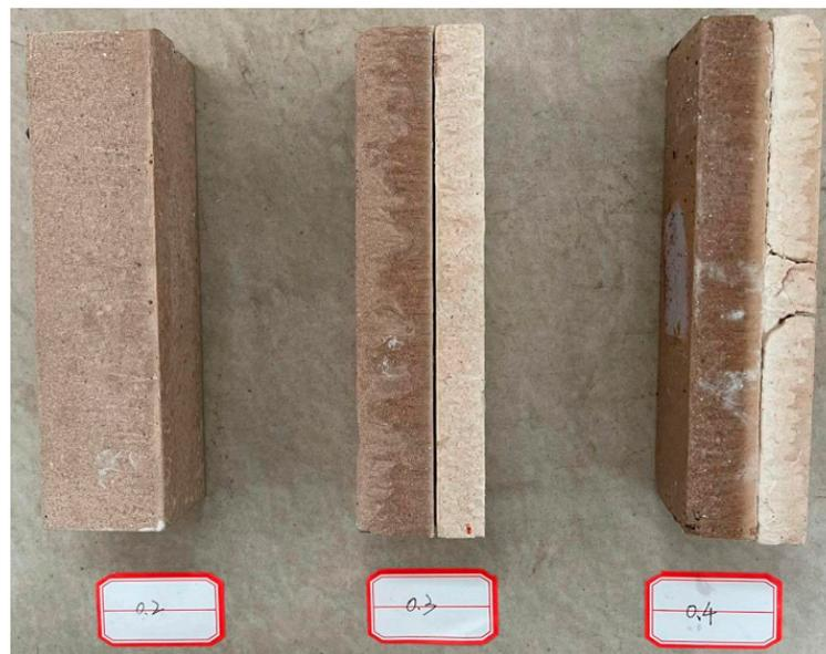
**Figure 6.** Appearances of MPC-TG pastes with different water-solid ratios.
