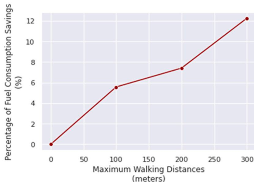
**Figure 5.** Percentage fuel consumption savings for each maximum walking distance.
