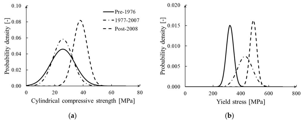
**Figure 14.** Possible definition of probabilistic distributions for material properties: concrete compressive strength (a) and steel yield stress (b).
