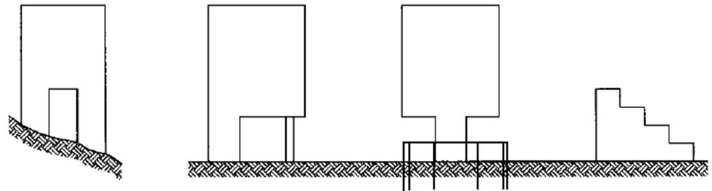
**Figure 4.** Geometric criticalities: examples of vertical irregularities (from [9]).
