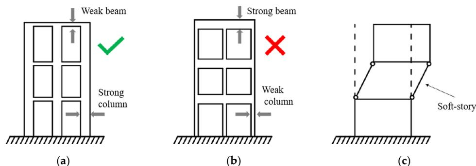
**Figure 7.** Structural details critical to the seismic response: example of presence (a) and lack (b) of hierarchy of strengths (capacity design) principles; a lack of hierarchy of strengths principles can lead to a soft-story failure mechanism (c).
