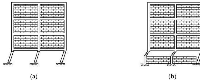
**Figure 5.** Construction criticalities: example of (a) non-uniform vertical distribution of infill walls, possibly leading to a soft-story failure mechanism, and (b) brittle failure due to short columns.
