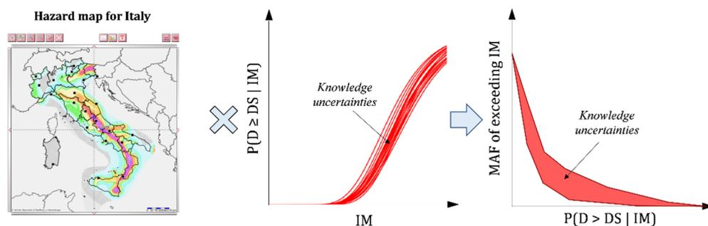
**Figure 21.** Example of seismic risk calculation in terms of Mean Annual Frequency, MAF, of exceeding a specific Damage State, DS, accounting for building knowledge uncertainties (hazard map for Italy available online: <http://esse1-gis.mi.ingv.it/>, accessed on 5 July 2022).
