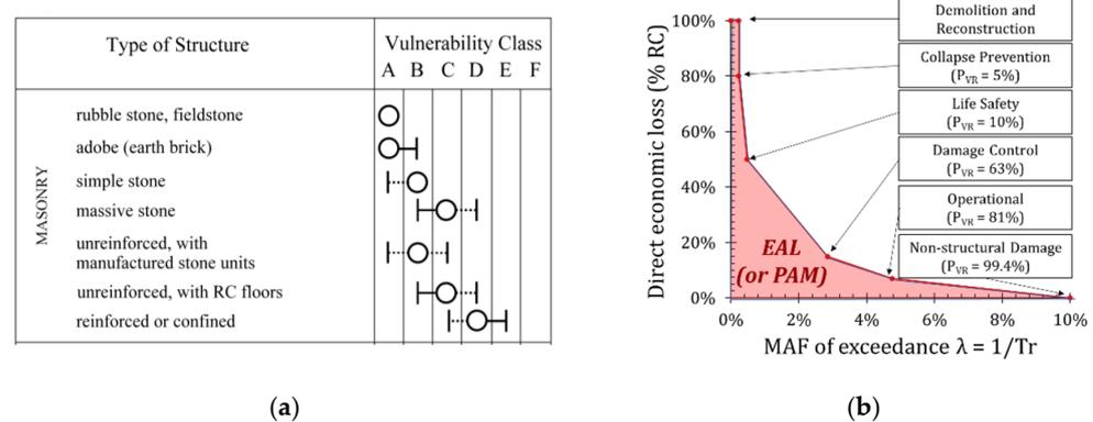
**Figure 9.** (a) Identification of the vulnerability classes for masonry buildings through the simplified approach based on the European Macroseismic Scale EMS-98 [28]; (b) EAL or PAM curve as defined in the SismaBonus guidelines [4].
