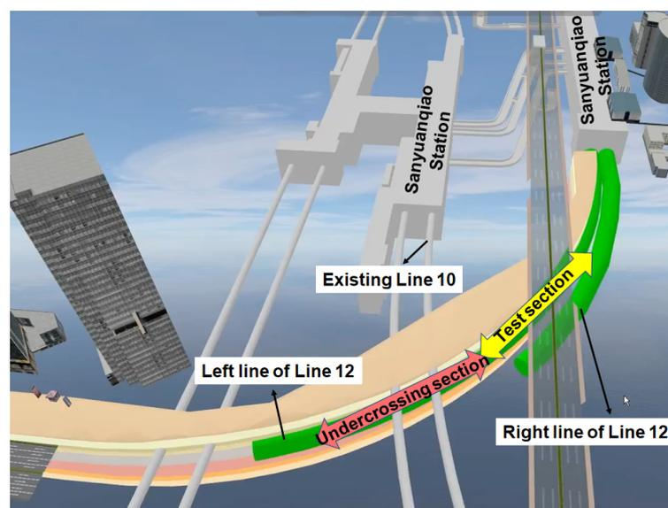
**Figure 3.** Layout of the test section and undercrossing section of tail grouting.
