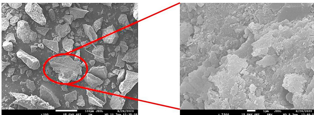
Figure 4. SEM images of dewatered aluminum Sludge.
