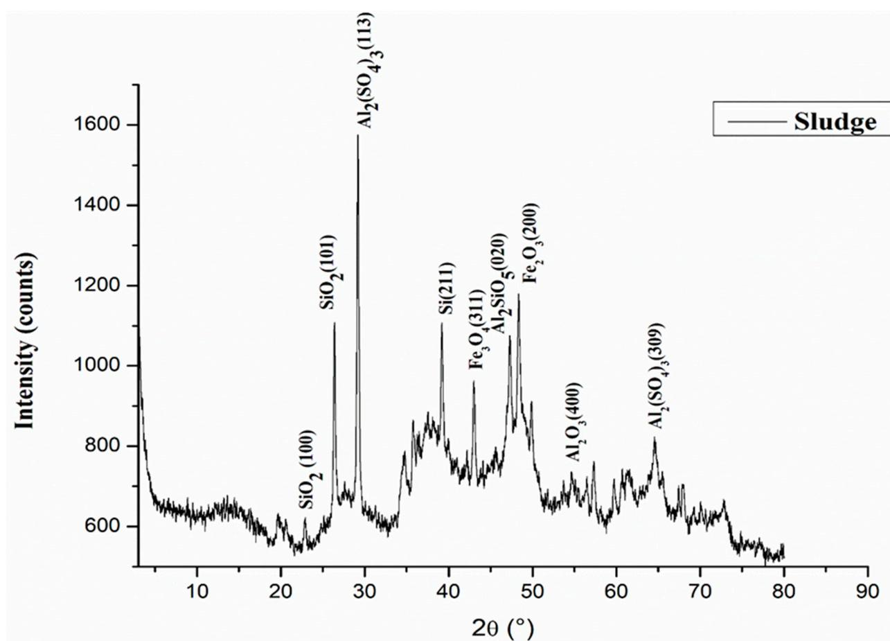
Figure 5. X-ray diffraction of Alum sludge.
