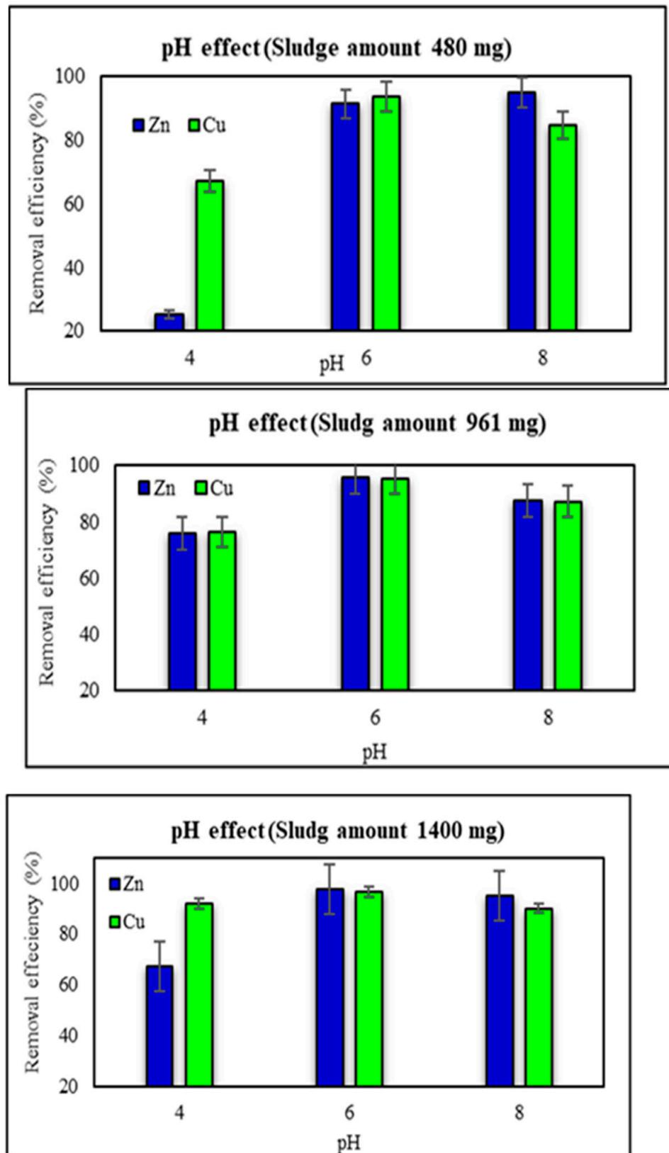
Figure 7. Effect of pH in Heavy metals removal using different sludge amounts.
