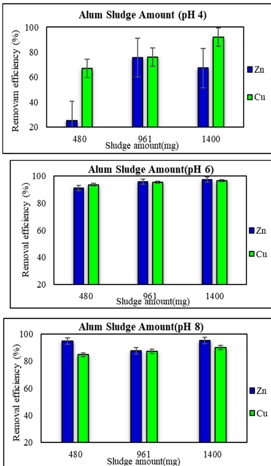
Figure 8. Effect of Sludge amount in Heavy metals removal in deferent pH mediums.
