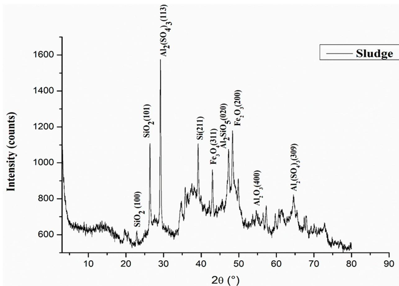
Figure 5. X-ray diffraction of Alum sludge.
