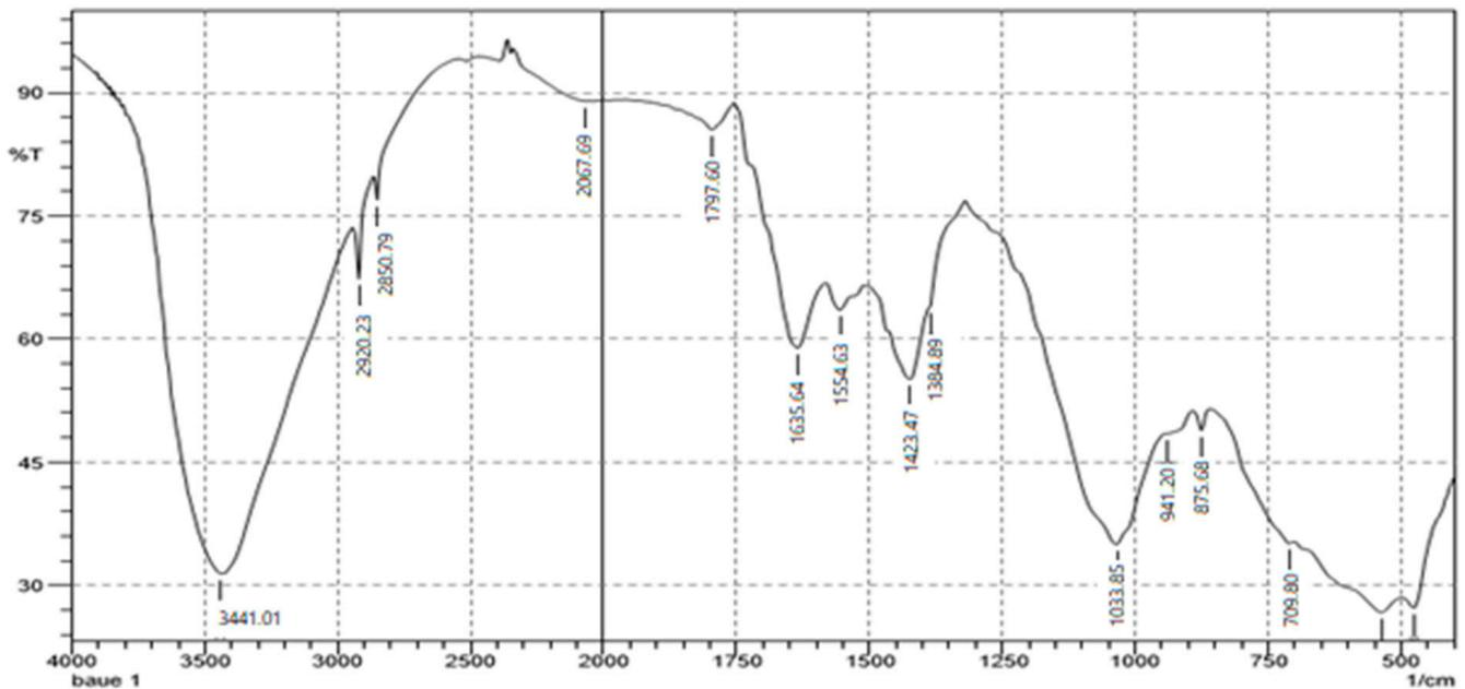
**Figure 6.** FTIR spectra of Alum sludge.
