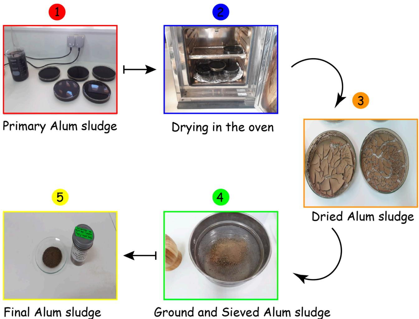
**Figure 3.** Schematic illustration of the preparation of Alum sludge sample.
