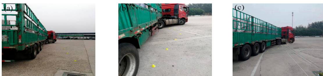
Figure 4. View boundary measurement for the rearview mirror: (a) The semitrailer truck starts to turn, and the rearview mirror has a maximum view; (b) the view in the rearview mirror gradually decreases; (c) the view of the rearview mirror reaches its minimum value during the turning process, and the rearview mirror fails considerably.
