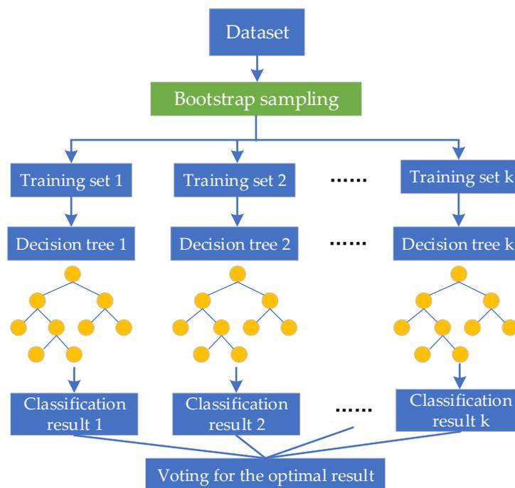
**Figure 3.** The flowchart of the RF model.
