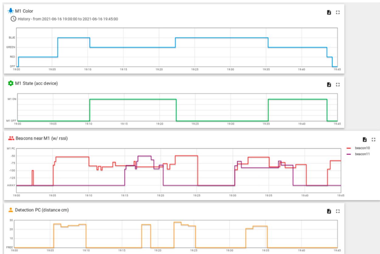
Figure 5. TB dashboard for M1: LED color (blue), machine state (green), BLE beacon signal strength for operators O10 (red) and O11 (purple), and the presence of an operator in front of the computer (yellow).
