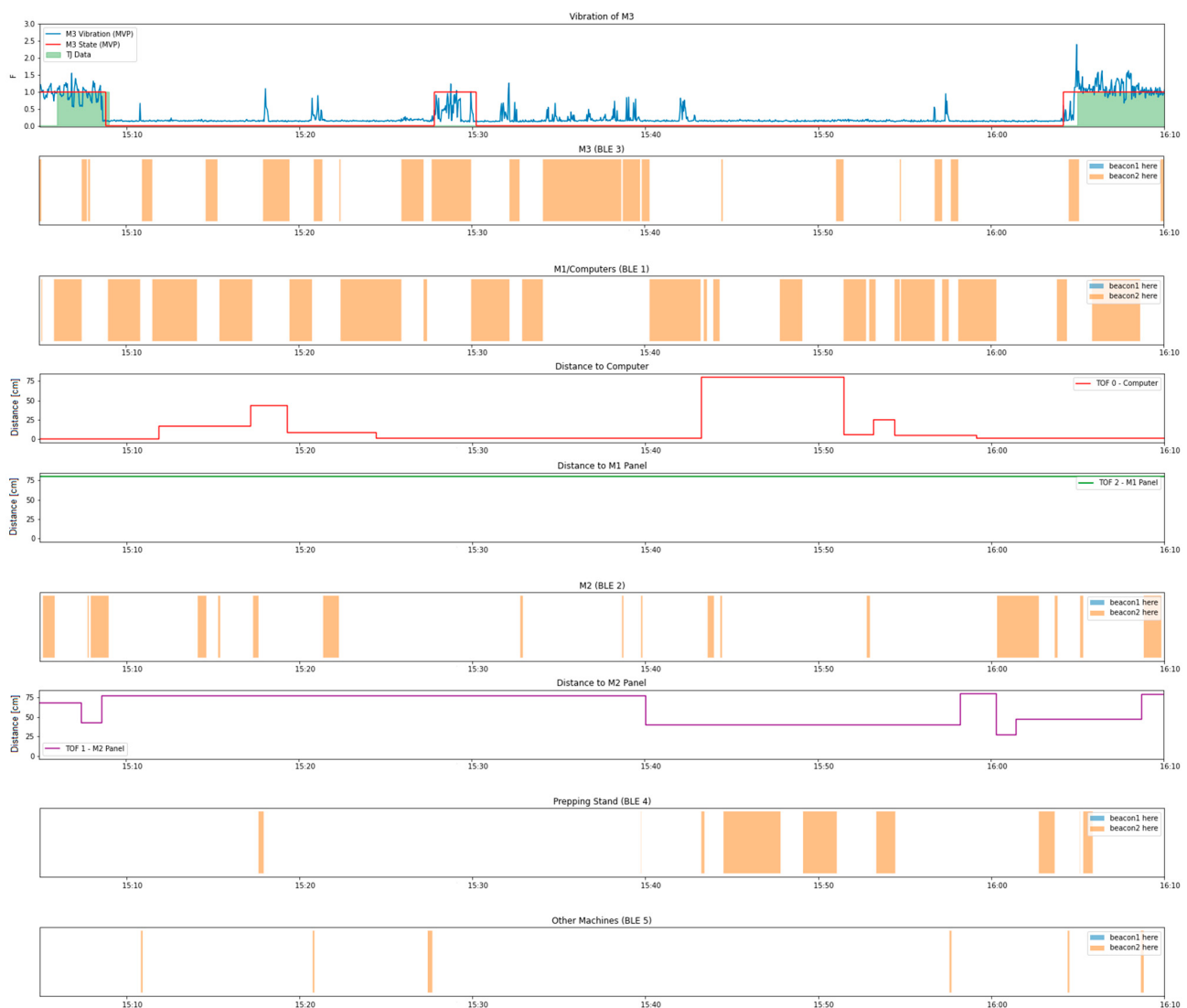
Figure 10. Dashboard of an M3 setup: vibration (blue), M3 state (red), spindle on (green), employees near M3 and M1 (employee 1 in blue and employee 2 in orange), someone in front of computers (red), someone in front of the M1 programming panel (green), employees near M2, someone in front of the M2 programming panel (purple), employees near the prepping stand and other machines.
