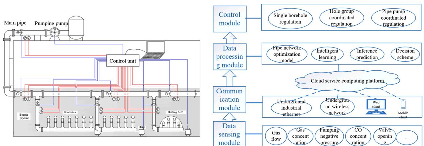
Figure 1. Structure and control principle of intelligent gas drainage [19].
