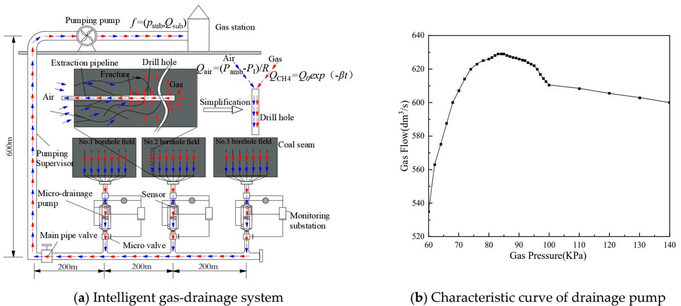
**Figure 5.** Intelligent gas-drainage system and the characteristic curve of drainage pump.
