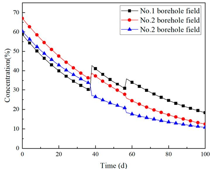
**Figure 9.** Variation curve of gas drainage concentration in each borehole field.
