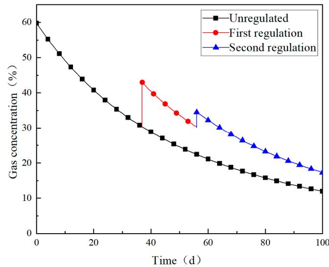
**Figure 8.** Change curve of outlet concentration of pipe network before and after regulation.
