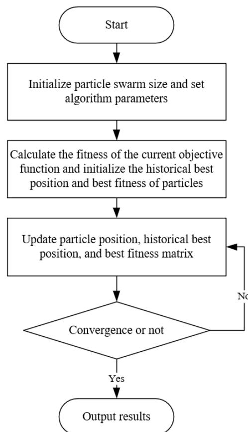
**Figure 4.** The calculation flow of PSO.
