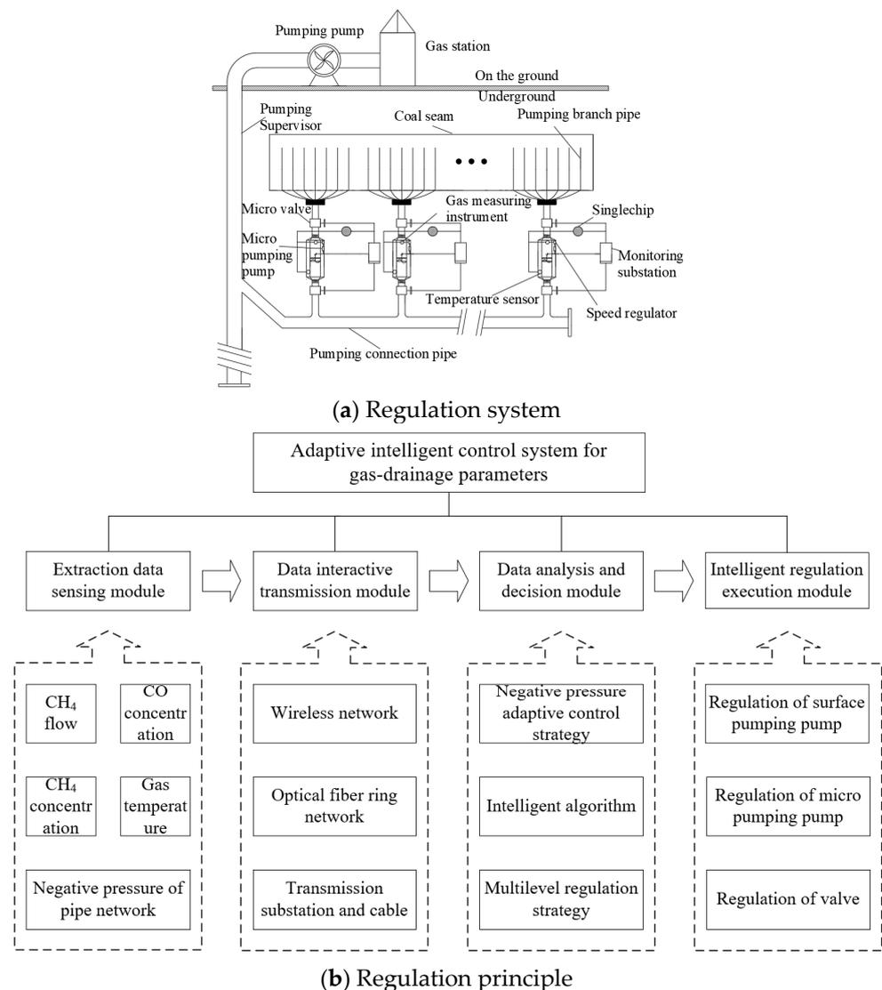
**Figure 2.** Adaptive control system of gas-drainage parameters.
