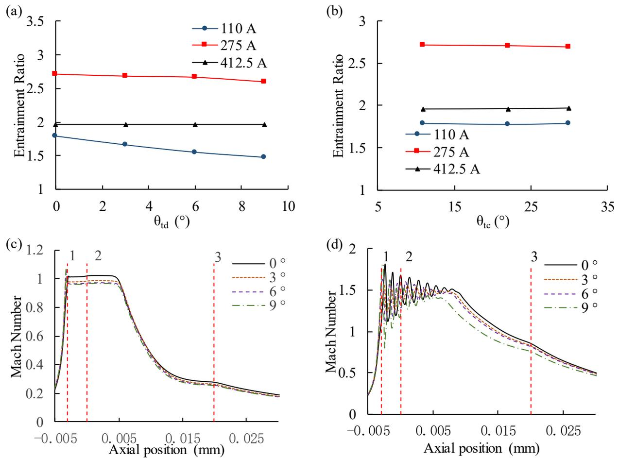
**Figure 7.** (a) Effect of nozzle convergence angle ( $\theta_{tc}$ ) on anode ejector; (b) Effect of nozzle divergent angle ( $\theta_{td}$ ) on anode ejector; (c) Mach number of different nozzle divergent angle at 110 A; (d) Mach number of different nozzle divergent angle at 275 A.
