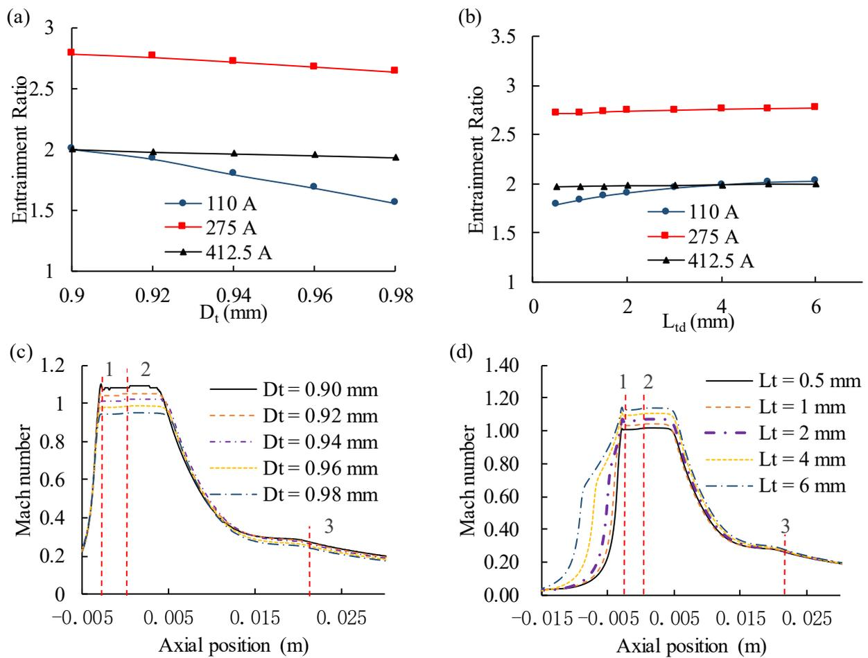
**Figure 6.** (a) Effect of nozzle throat diameter ( $D_t$ ) on anode ejector; (b) Effect of nozzle throat length ( $L_{td}$ ) on anode ejector entrainment ratio; (c) Mach number of different nozzle throat diameter at 110 A; (d) Mach number of different nozzle throat length at 110 A. (Dash red lines 1, 2, and 3 in figure are the nozzle exit, the mixing tube inlet and the mixing tube exit, respectively.)
