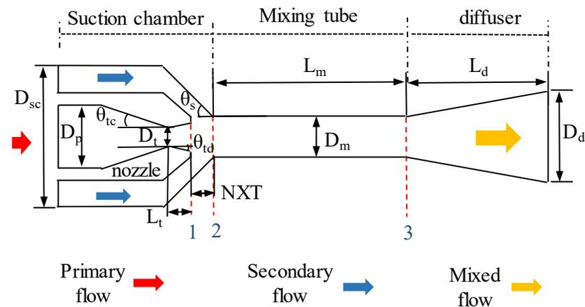
Figure 2. Ejector schematic.
