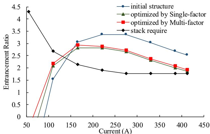
**Figure 16.** Comparison of initial ejector with optimized ejector.
