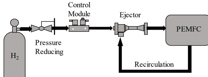
**Figure 1.** Diagram of the recirculation system for a PEMFC using an ejector.
