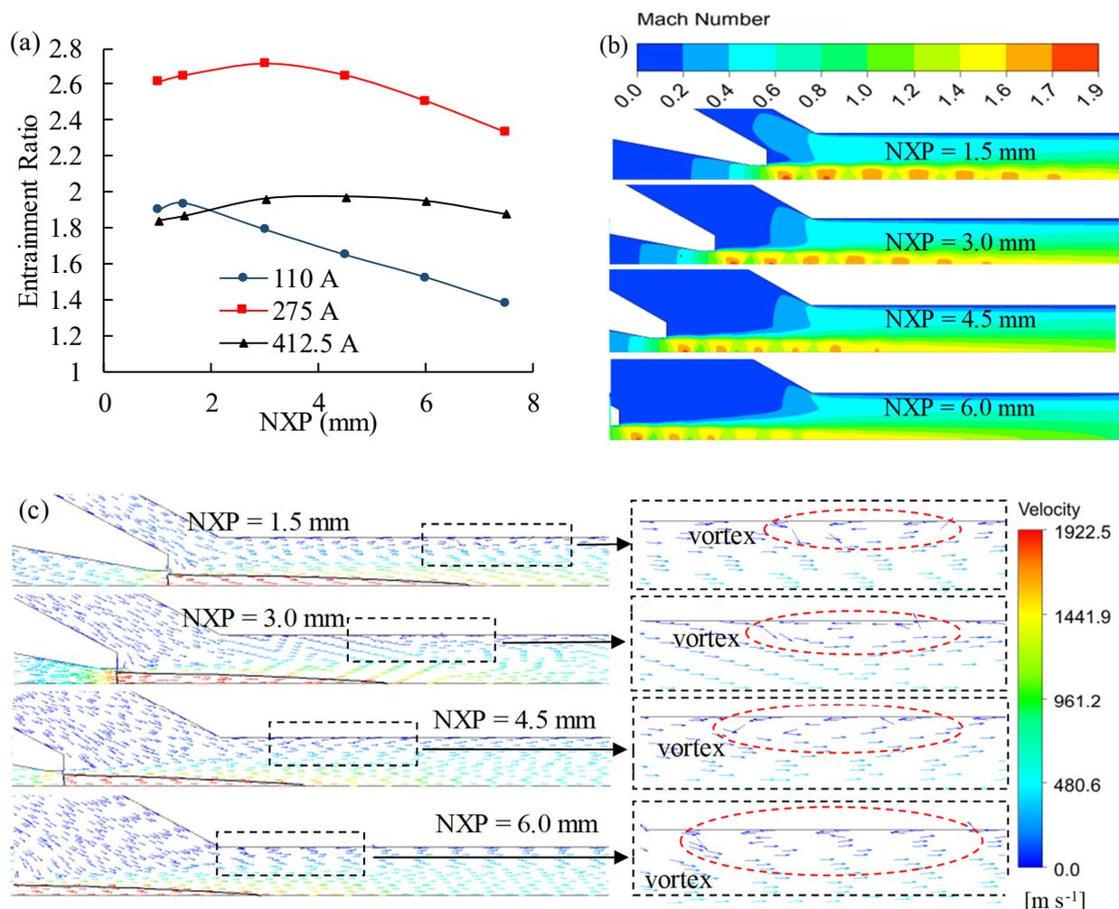
**Figure 8.** Effect of NXP on PEMFC ejector. (a) Entrainment ratio; (b) Mach number of different NXP at 275 A; (c) Velocity vector diagrams of different NXP at 110 A. (The black box shows an enlarged view of the local flow. The red circle represents the vortex generation zone.)
