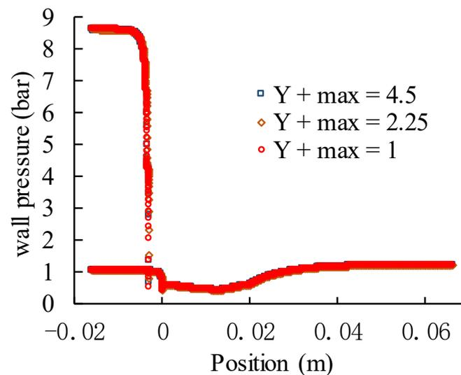
**Figure 4.** Change of wall pressure with different  $y^+$ .
