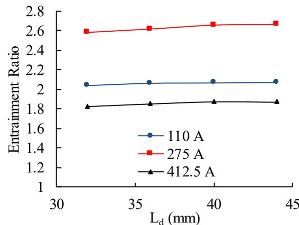
Figure 12. Effect of diffuser length ( $L_d$ ) on PEMFC ejector entrainment ratio.
