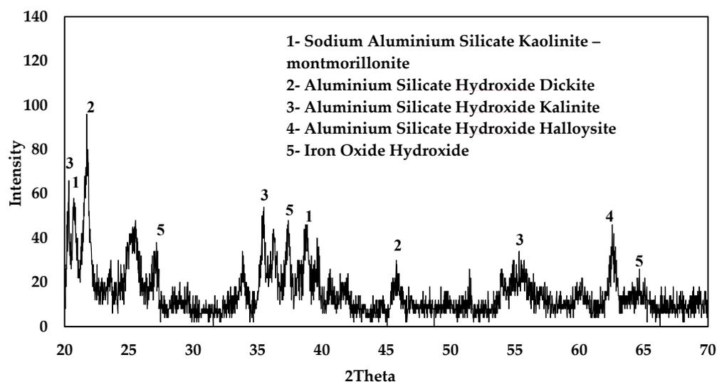
**Figure 2.** X-ray-diffraction pattern of lateritic soil.
