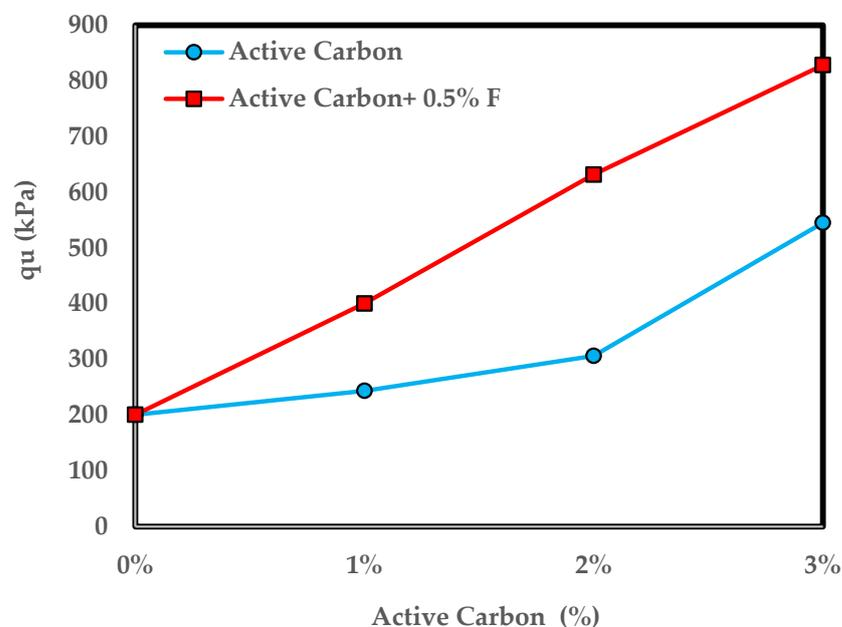
**Figure 12.** Compressive strength (UCS) for different AC contents.
