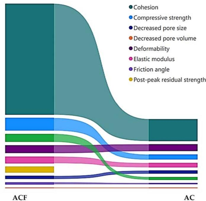
**Figure 16.** Scheme of effect-activated carbon and coir fiber on geotechnical parameters.
