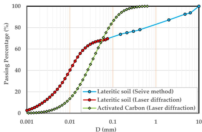
**Figure 1.** Particle-size analysis of soil and AC.
