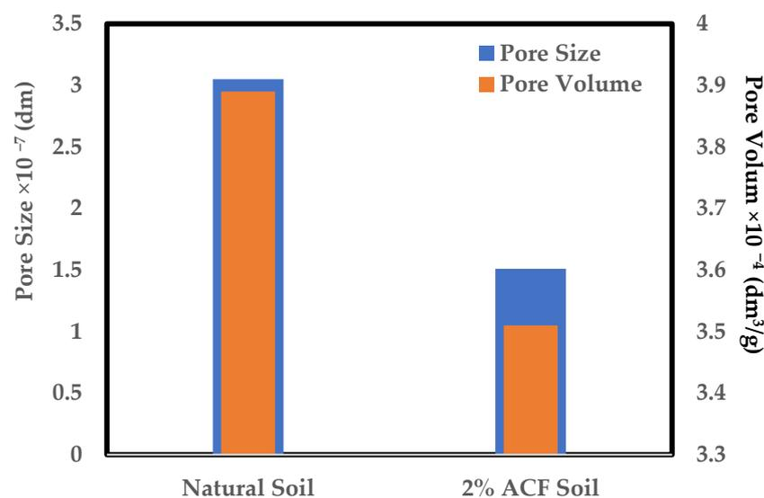
Figure 11. Pore volume, surface area, and pore size of lateritic soil and 2% ACF soil.
