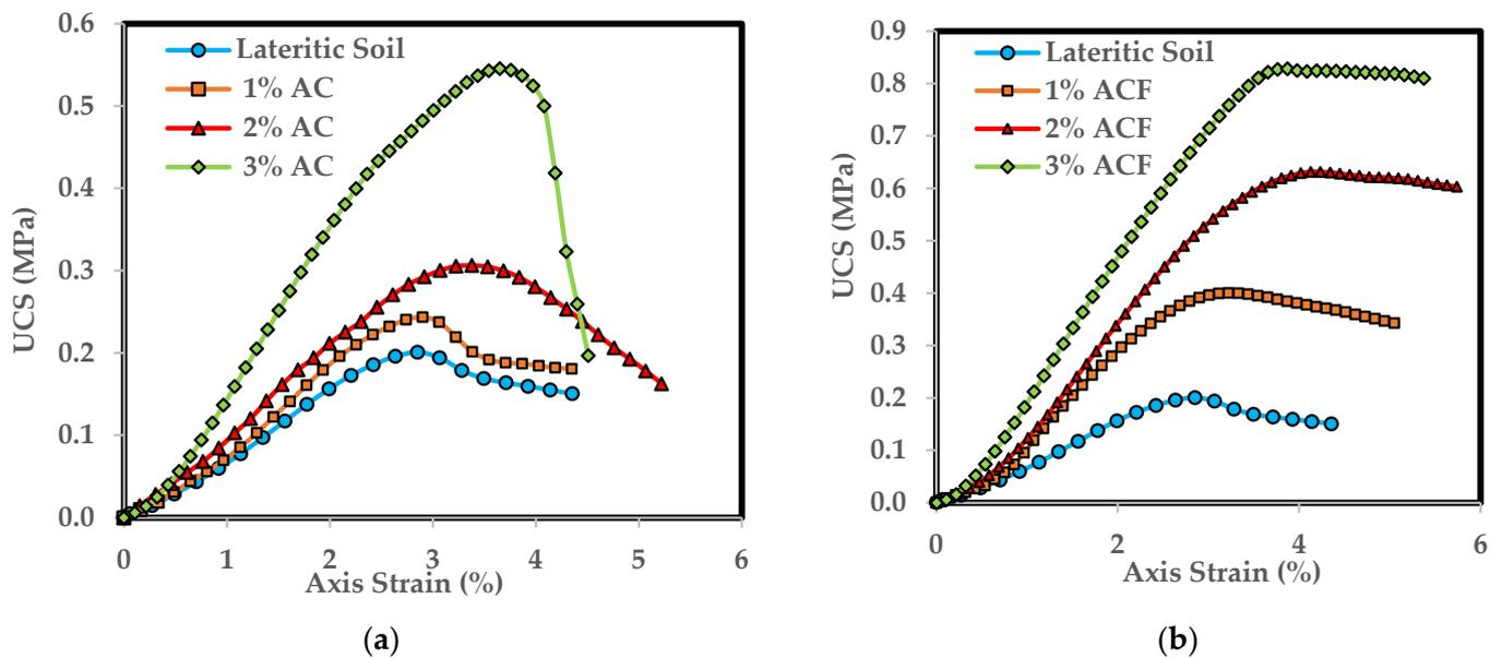
**Figure 6.** UCS results for (a) AC specimens and (b) ACF specimens.
