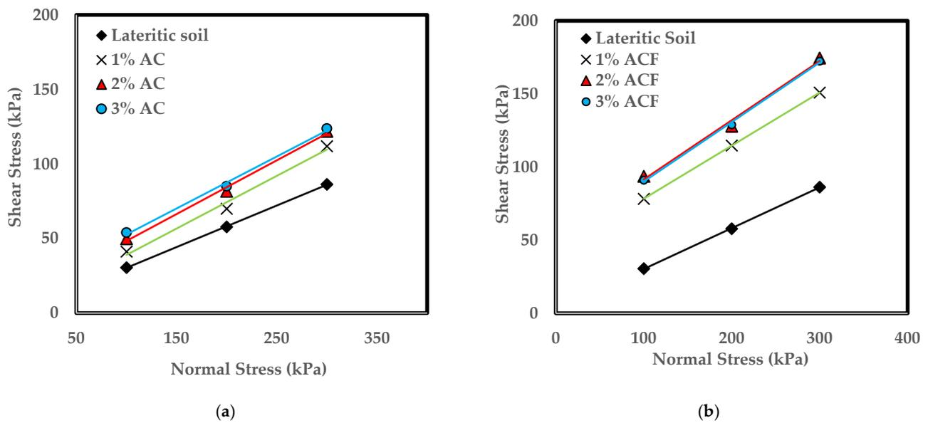
**Figure 13.** The relationship between peak shear strength and normal stress lateritic soil treated with (a). various AC content and (b) various ACF content.
