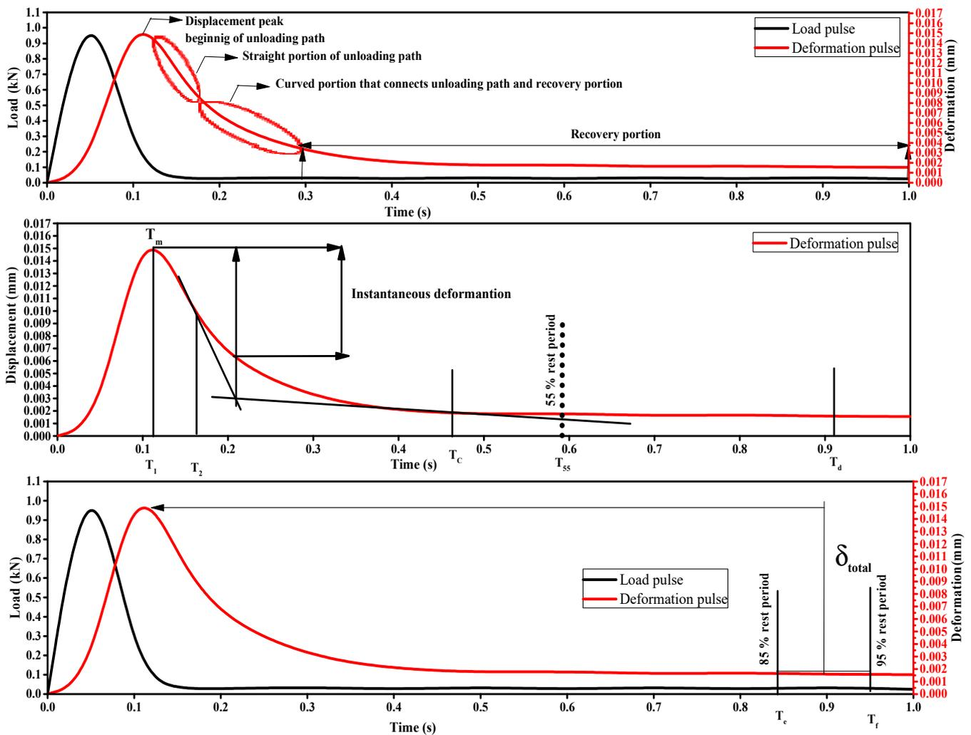
**Figure 2.** Typical load-time and deformation-time plots for a single cycle with time parameter explanation during  $M_R$  tests, as per ASTM D7369.
