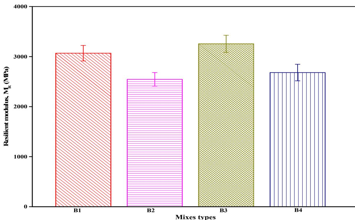
**Figure 5.** Resilient modulus of modified and unmodified asphalt mixes (B1–B4).
