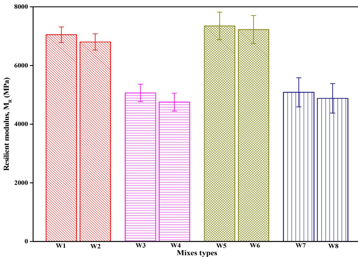
Figure 3. Resilient modulus of modified and unmodified asphalt mixes (W1–W8).
