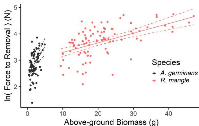
**Figure 5.** Linear regression models with 95% confidence intervals for anchoring force of *Rhizophora mangle* L. and *Avicennia germinans* (L.) L. measured in field pull tests as a function of above-ground biomass.
