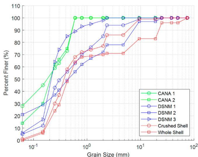
**Figure 7.** Grain size distributions of field sediments by site and laboratory sediment treatments.
