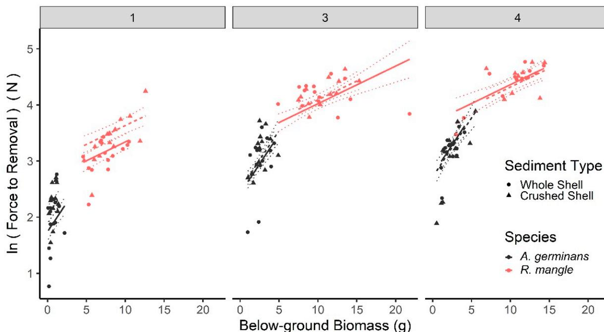
**Figure 8.** Linear regression model with 95% confidence intervals of 1-, 3- and 4-month old *Avicennia germinans* (L.) L. and *Rhizophora mangle* L. anchoring force measured in laboratory pull tests as a function of below-ground biomass.
