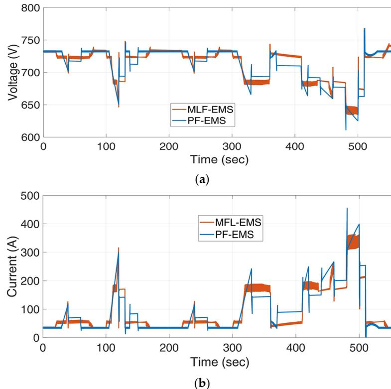
**Figure 17.** Fuel cell voltage and current profile in FCHPS for proposed MFL-EMS and traditional method. (a) Voltage. (b) Current.
