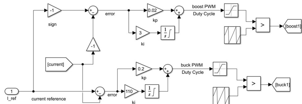
Figure 5. Bidirectional DC-DC controller model.
