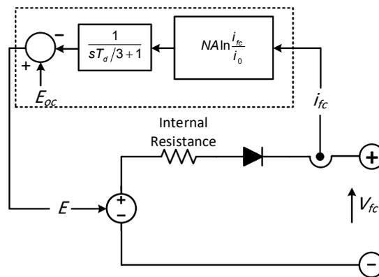
Figure 2. PEMFC equivalent circuit.
