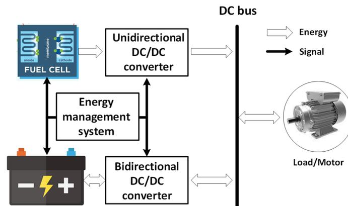
**Figure 1.** The energy flow diagram of the proposed hybrid locomotive topology.
