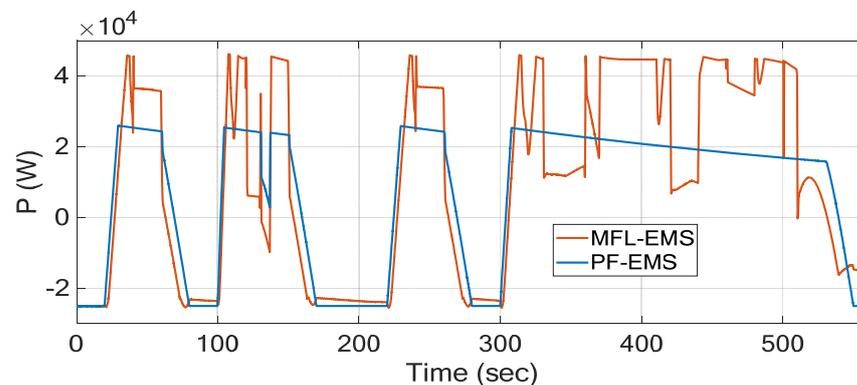
Figure 14. Battery power profile for FCHPS for proposed MFL-EMS and traditional method.
