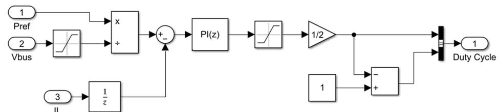
Figure 4. Boost DC-DC converter control block model.
