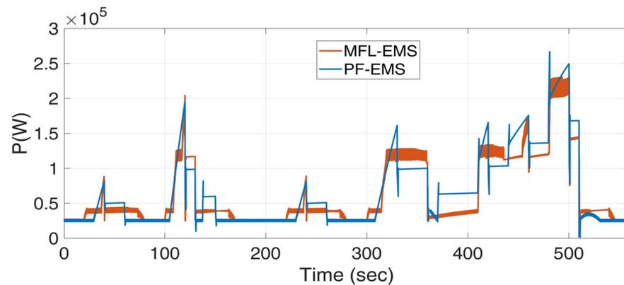
Figure 12. Fuel Cell power with proposed MFL-EMS and conventional PF-EMS.
