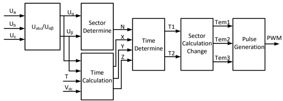
Figure 6. SVPWM basic diagram.
