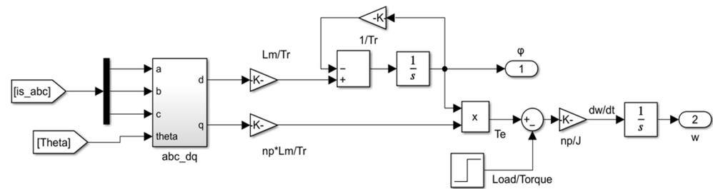
Figure 7. Three-phase asynchronous motor model in the locomotive.
