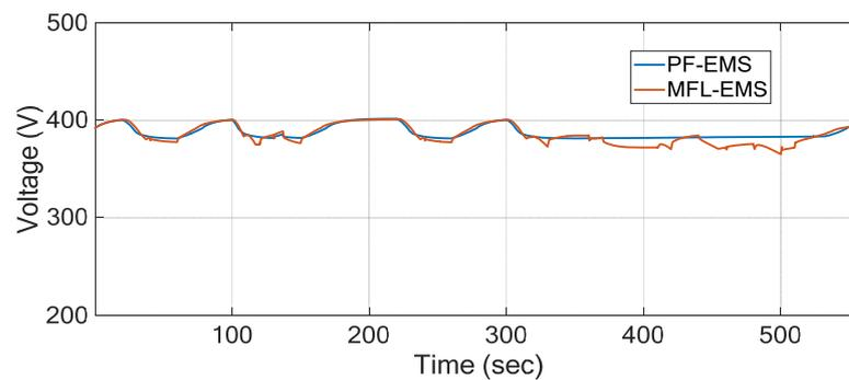
**Figure 16.** Battery voltage in the FCHPS for proposed MFL-EMS and traditional method.
