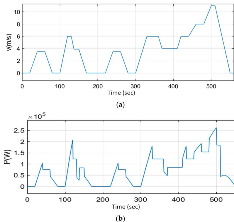
**Figure 11.** Driving cycle features of the locomotive in the proposed system. (a) Speed. (b) Required power.
