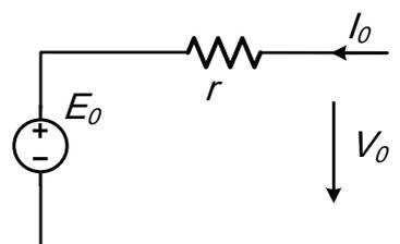
Figure 3. Equivalent circuit of the battery.
