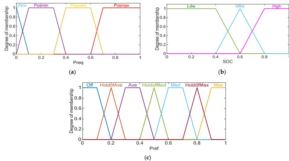
**Figure 9.** Fuzzy membership functions. (a) membership function of fuel cell power as input. (b) membership function of SOC as input. (c) membership function of reference power as output.
