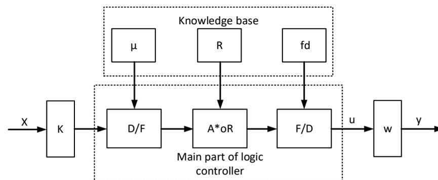
Figure 8. Structure of the fuzzy controller.
