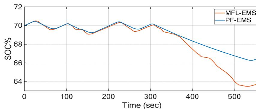
Figure 15. Battery SOC% in the FCHPS for proposed MFL-EMS and traditional method.
