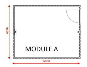
Figure 21. Module A obtained by the combination on the long side of 2 containers TOP 20'.
