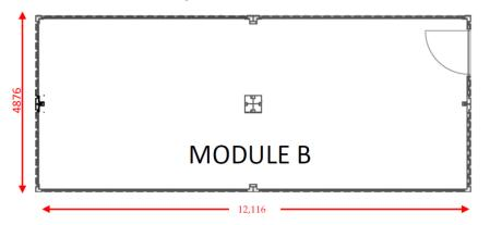
Figure 22. Module B obtained by the combination of 4 containers TOP 20'.
