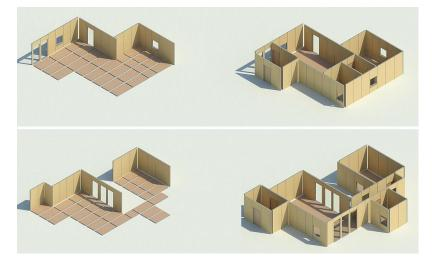
Figure 8. Installation diagram of the panels.
