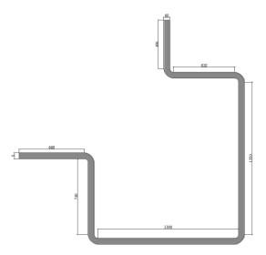
Figure 27. Construction details of the locking package.
