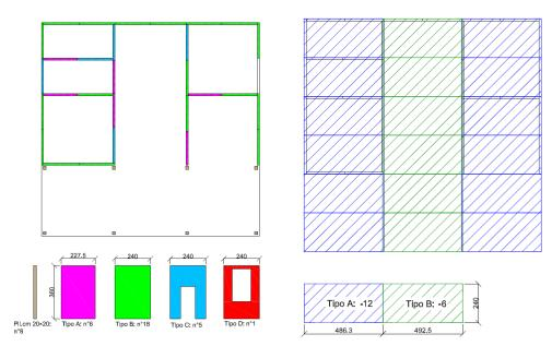
Figure 19. Abacus of the wall of the multifunctional module.
