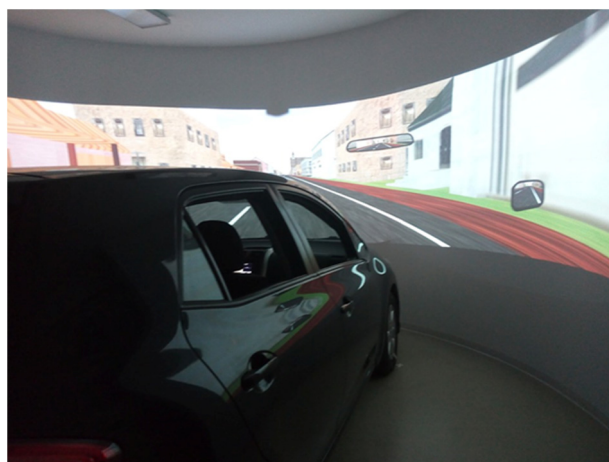
Figure 1. LassTRE virtual reality driving simulator.
