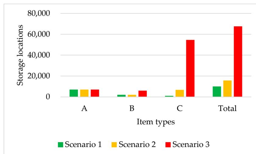
**Figure 6.** Needed capacity (in cases' storage locations) for Warehouse 2 for the three scenarios.
