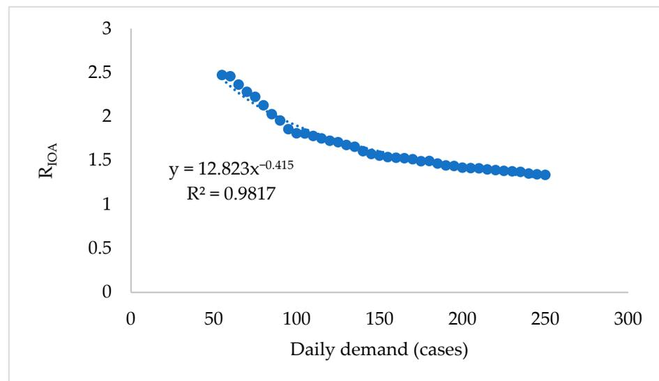
Figure 3. Ratio between output and input pallets of A items for WH1 (scenario 2).
