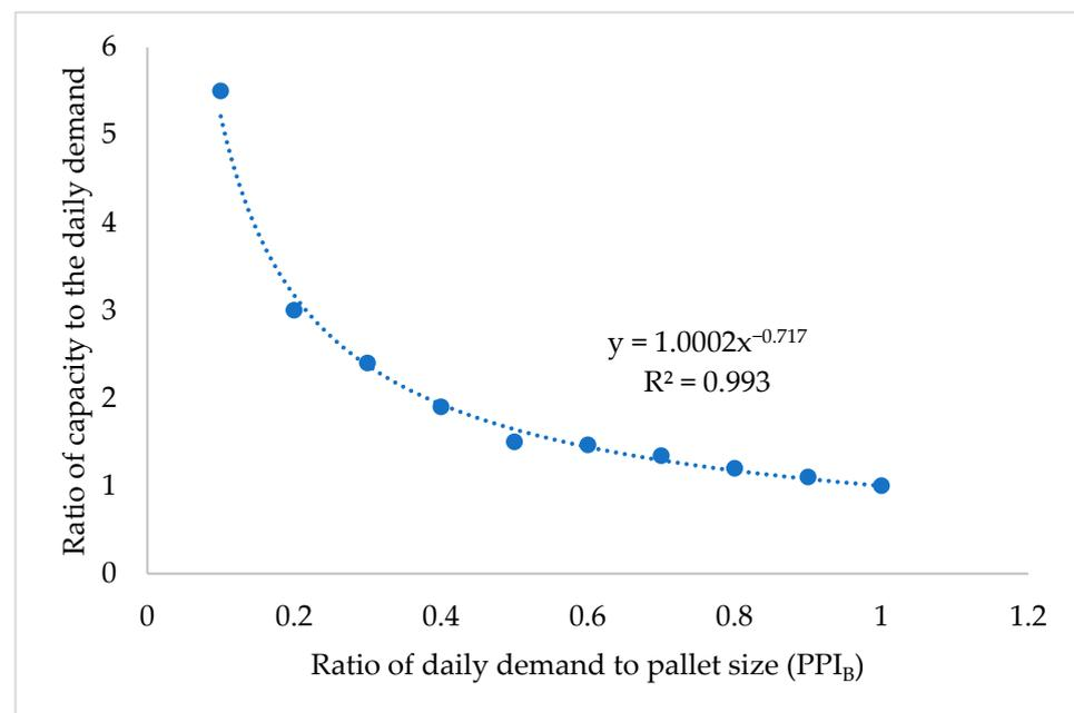
**Figure 4.** A way to find the needed capacity of WH2 for B items (for scenario 3).
