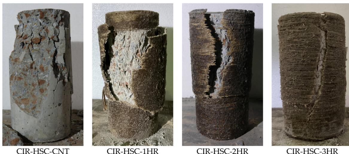
**Figure 5.** Ultimate failure modes.
