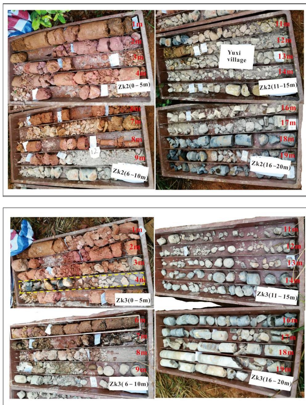
**Figure 4.** Drilling core samples from three boreholes (ZK1, ZK2, ZK3).
