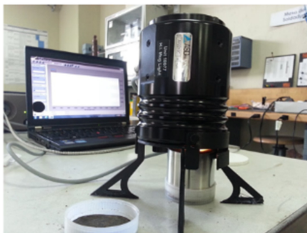
Figure 4. Location of cylinder with respect to HiBrite MudLight device on support.
