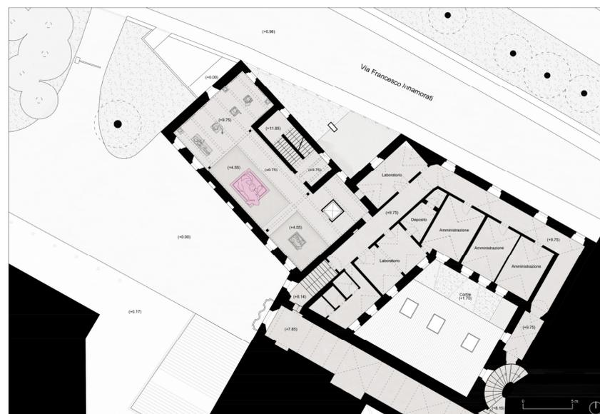
**Figure 9.** Extract of the proposed project. Plan of the second floor of plaster casts gallery of the University of Perugia, object of the emptying and, through a new steel structure, of architectural redevelopment.
