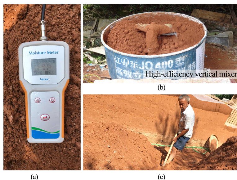
Figure 5. Instruments and construction materials used for testing materials' moisture content. (a) Soil moisture measuring instrument. (b) High efficiency vertical mixer. (c) Traditional rammed earth materials.
