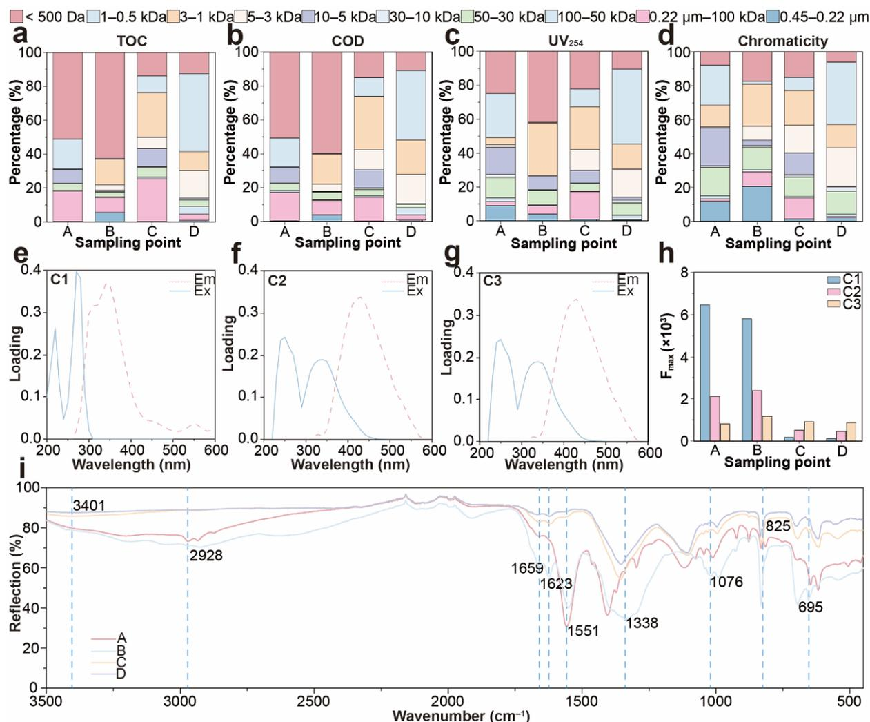
**Figure 4.** The transformation of DOMs in the co-digestion wastewater revealed by (a–d) molecular weight cut-off, (e–h) 3D-EEM, and (i) FT-IR.
