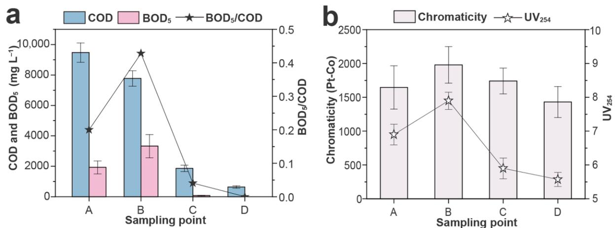
**Figure 3.** The variation in (a) COD, BOD<sub>5</sub>, (b) UV<sub>254</sub>, and chromaticity of the co-digestion wastewater along the treatment process.
