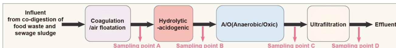
**Figure 1.** Process flow diagram and sampling points of the full-scale anaerobic digestion wastewater treatment facility.
