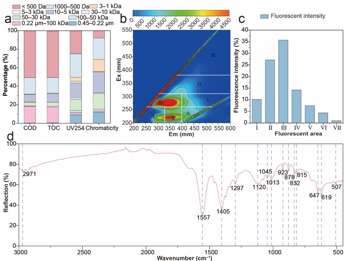
**Figure 2.** The characterization of DOMs in the co-digestion wastewater of sewage sludge and food waste: (a) molecular weight distribution; (b) 3D-EEM spectra; (c) the distribution of fluorescence regional integration; (d) FT-IR spectra.
