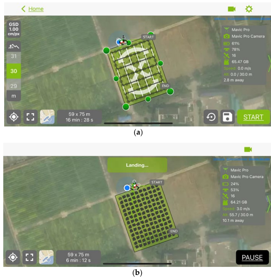
Figure 2. UAV image collection. (a,b) is the flight planning mission in Pix4Dcapture: (a) is the start of the mission, and (b) is the end of the mission.
