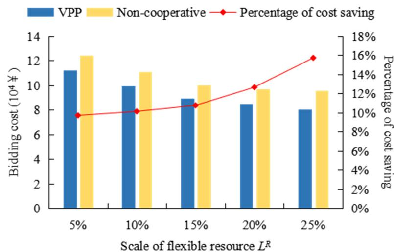
Figure 12. Cooperative benefits of VPP under different flexible load scales.
