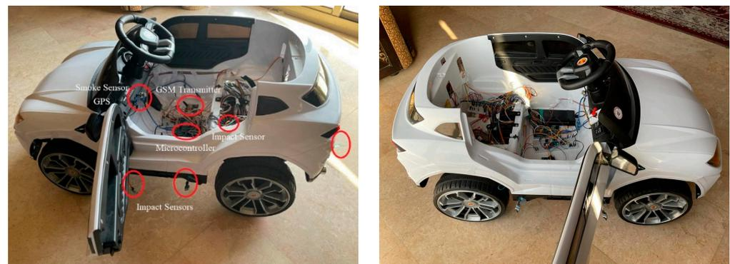
**Figure 6.** Hardware setup of the accident detection and classification system.
