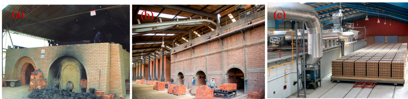
Figure 2. Relative high-tech brick kilns: (a) zig-zag kiln; (b) Vertical shaft brick kiln; and (c) Tunnel kiln.
