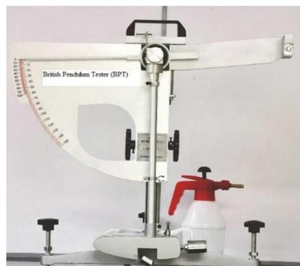
**Figure 3.** British Pendulum Tester device used for skid resistance test.
