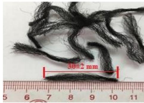
**Figure 1.** Waste polypropylene fibres from the carpet industry.
