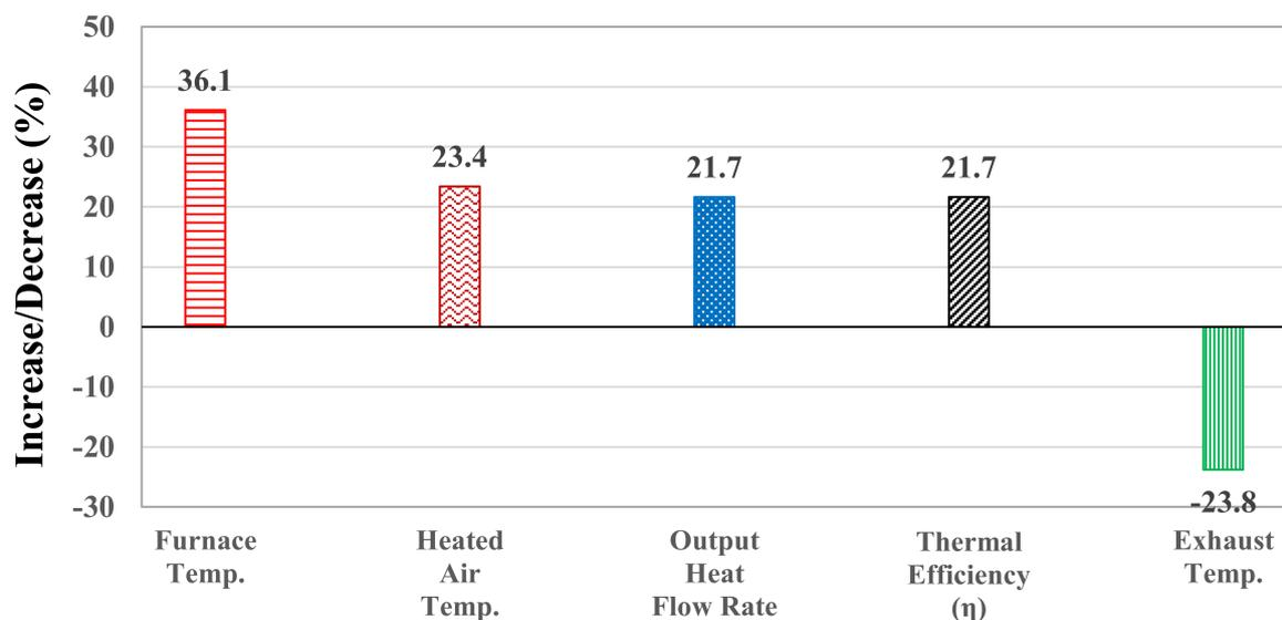
**Figure 7.** Improvements in various parameters after the modification of the biomass furnace.
