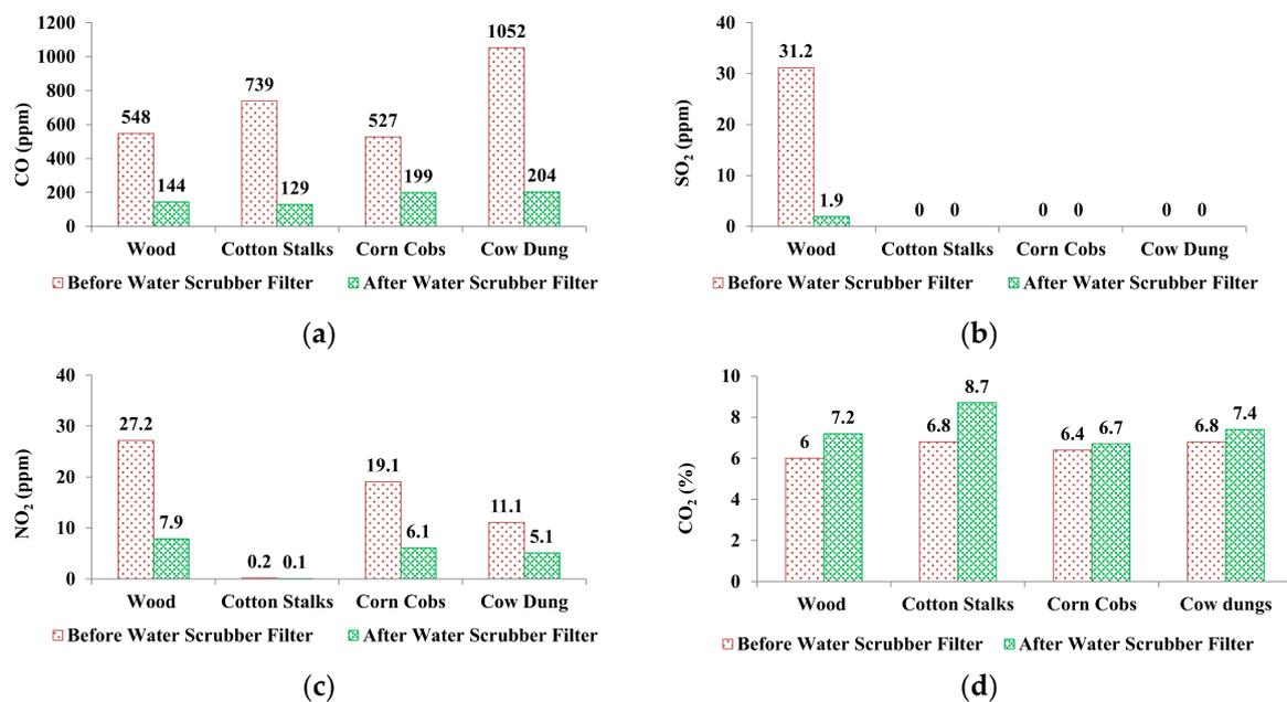
**Figure 8.** Flue gas concentrations of different biomass fuels before and after the water scrubber. (a) Carbon monoxide (CO). (b) Sulphur dioxide (SO<sub>2</sub>). (c) Nitrogen dioxide (NO<sub>2</sub>). (d) Carbon dioxide (CO<sub>2</sub>).
