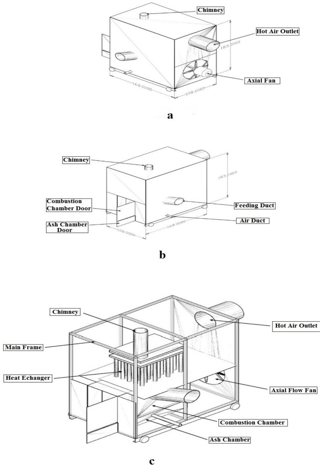
Figure 1. Schematic diagram of biomass furnace (a) back view (b) front view, and (c) cross-sectional view.
