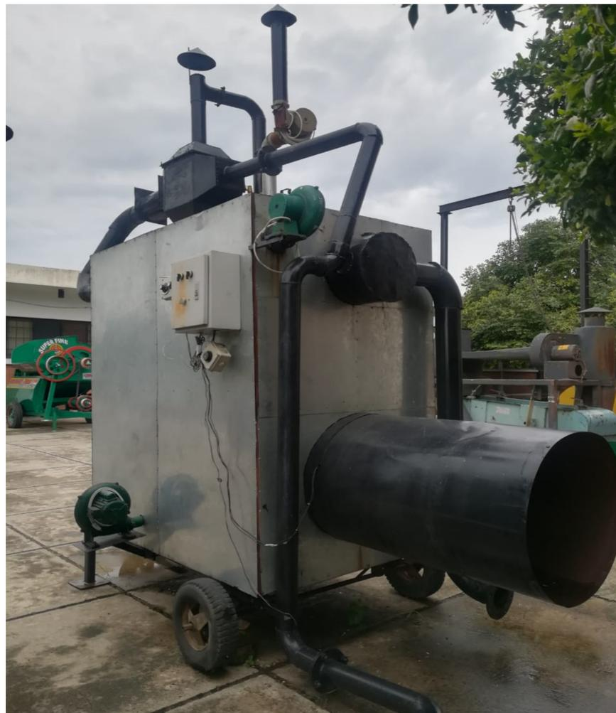
**Figure 6.** Side view of the modified biomass furnace.
