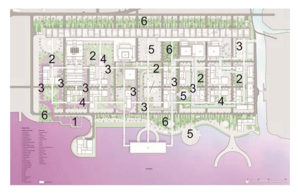
**Figure 4.** Masterplan Lifelong learning: 1. Floating residues filtration, 2. Biotopes, 3. Canals, 4. Detention Ponds, 5. Wet/dry islands, 6. Infiltration Zones (bio-swales), designed by: Tianning Ren, Yulin Zhang, Yixuan Chen, Jiamei Song, 2020.
