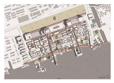
**Figure 11.** Masterplan coexistence agreement, a selection of strategies' locations: 3. Canals, 4. Detention ponds, 6. Infiltration zones, 9. Green roofs. Designed by: Zhengyou Chen, Tiancheng Kang, Yuhang Tao, Hanwen Xu, 2020.
