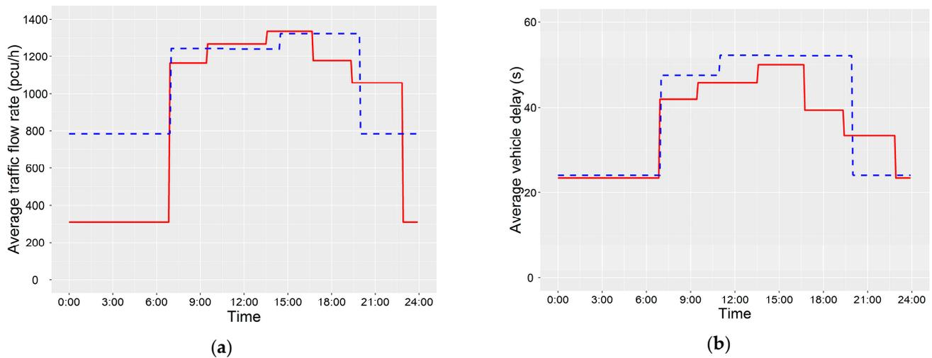
**Figure 4.** Evaluation indices between Plan A (solid red line) and Plan B (dashed blue line). (a) Average traffic flow rate, (b) Average vehicle delay.
