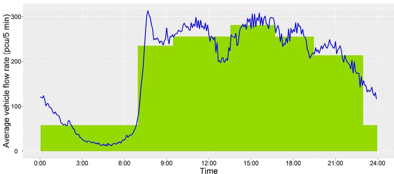
**Figure 3.** The clustering results of cyclic weighted  $k$ -means method.
