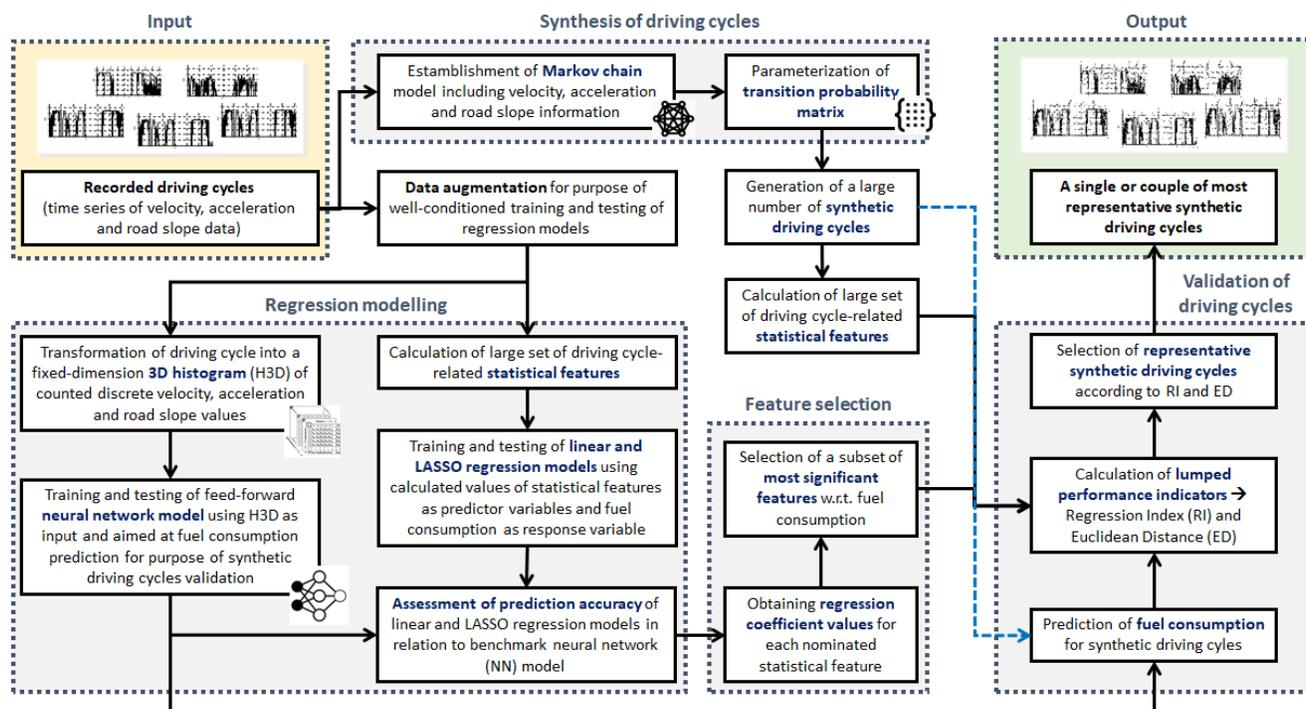
Figure 1. Flowchart of the overall proposed methodology.
