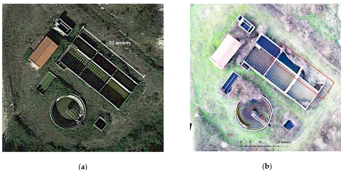
Figure 10. The wastewater treatment plant that was constructed in 1999 was captured (a) by the satellite image from Google Maps in 2016; (b) by the orthomosaic generated in Pix4D in 2020. The destruction of its walls is visible in the NE water tanks (in the red square) that are being filled with sediment.
