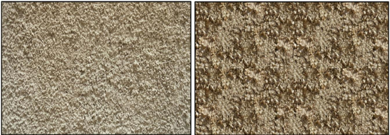
**Figure 6.** Rough texture with different concentration of palm particles aggregate.
