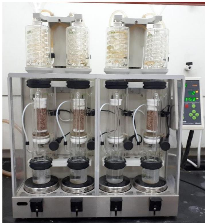
**Figure 1.** Fat extraction apparatus (Soxhlet apparatus).
