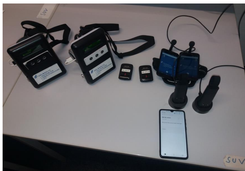
Figure 2. Overview of pollution (air and noise) sensing materials and additional accessories (GPS, temperature and humidity measurement devices) when meeting citizen science projects in Leipzig, Germany. Low-cost sensors used at Helmholtz UFZ are described in [19].
